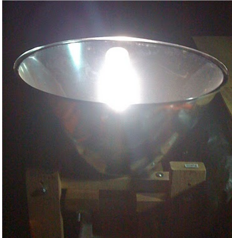
Figure 4: A 1000W high pressure sodium lamp with a 22 inch aluminum reflector.
