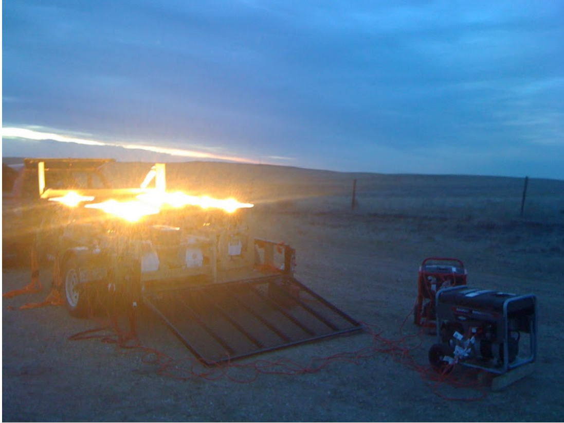
Figure 5: Seven (1000W) high pressure sodium lights in the utility trailer and the two generators used to power the lights in the field.
