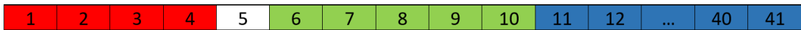
Figure 3.18: A UDP packet sent by X-Plane to Simulink. Bytes 1-4 contain the Header, byte 5 is a software internal use byte, bytes 6-10 contain the data label, and bytes 11-41 contain the estimated aerodynamic variables.
