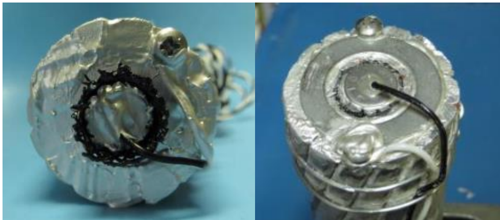
Figure 36: Simple electrical connections for short-term corrosion testing. The connections will be covered with silicone RTV before exposure to the corrosive environment.
