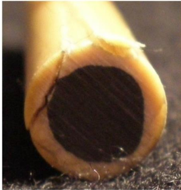
Figure 3 (repeated): Cracks in the ACCC conductor corrosion barrier caused by Aeolian vibrations (high cycle fatigue) (Burks, Armentrout et al. 2011).
