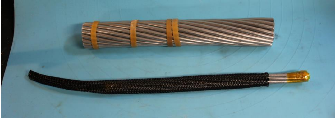
Figure 40: The core partially covered with the polyester mesh.
