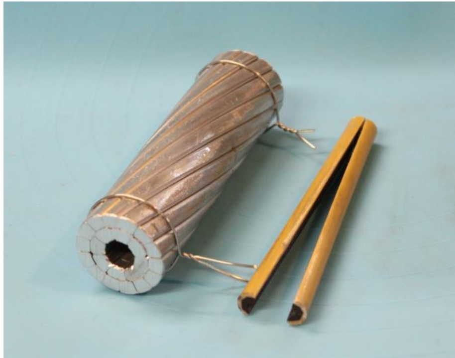
Figure 53: The split core (right) and the surrounding aluminum strands (left)
