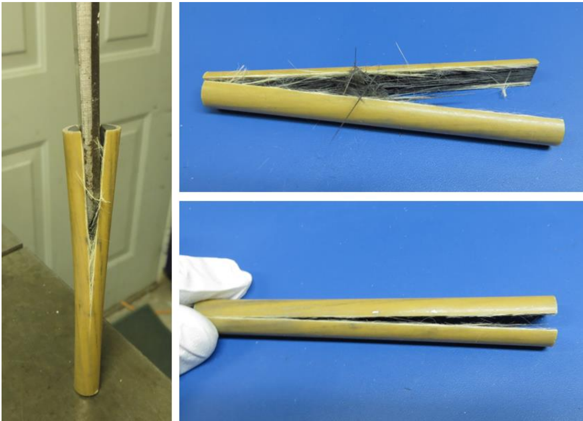
Figure 52: Splitting of the ACCC core to simulate damage.
