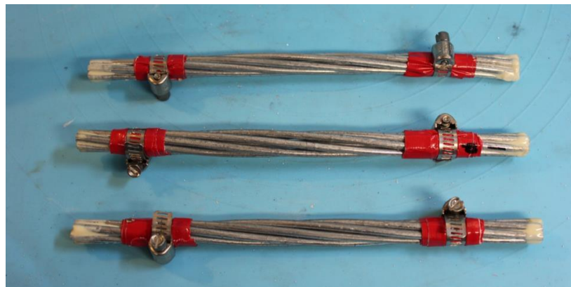
Figure 39: Ends dipped in fast-curing epoxy.
