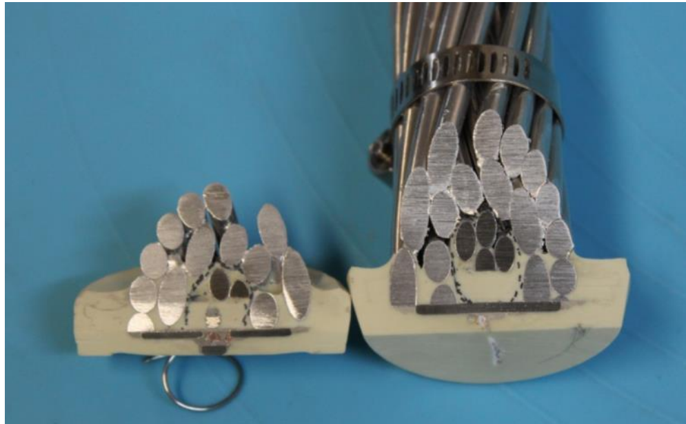
Figure 48: Sectioned view of the electrical connection to the aluminum strands.
