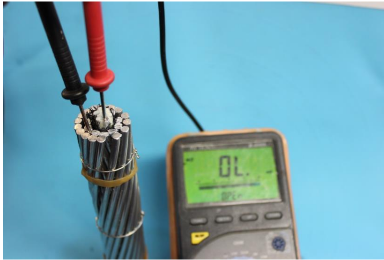
Figure 50: Control of continuity.
