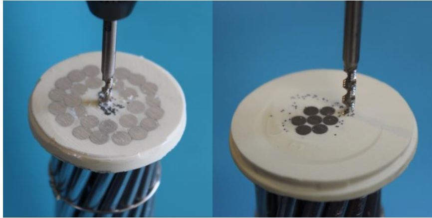
Figure 44: Holes are drilled and tapped.
