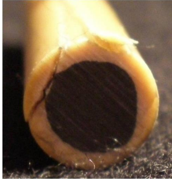
Figure 3: Cracks in the ACCC conductor corrosion barrier caused by Aeolian vibrations (high cycle fatigue).
