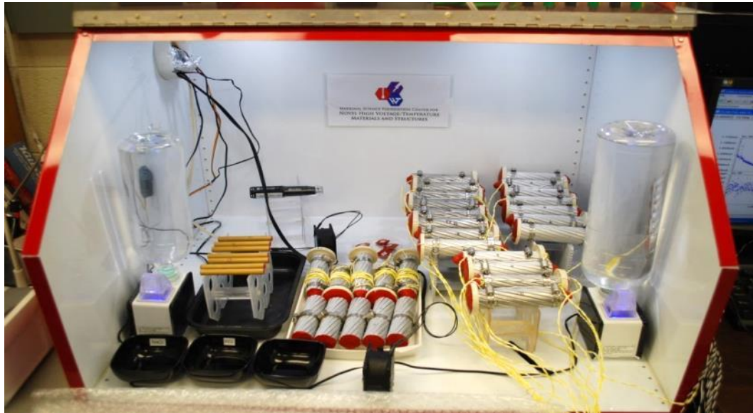
Figure 147: Validation samples in the humidity chamber.
