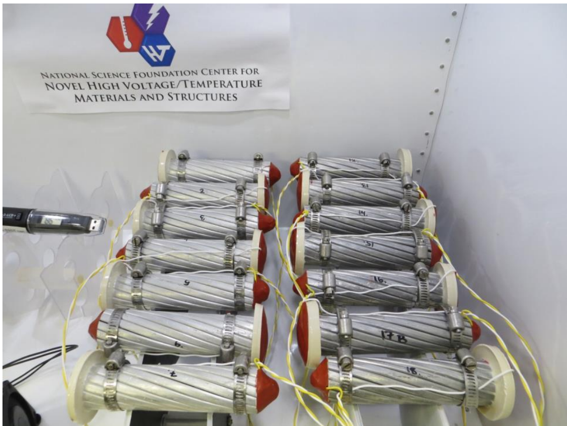
Figure 67: Finished ACCC samples in the humidity chamber.
