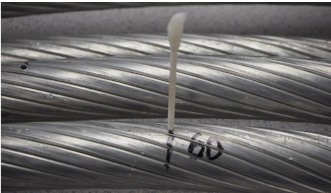
Figure 173: Paper rod soaked in NaCl solution inserted to make electrical contact between the Al and the CFRP.
