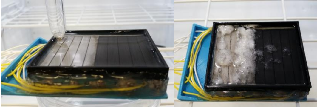
Figure 152: \text{Al}(\text{OH})_3 gel formation on a coplanar aluminum-graphite couple. Left) Start; Right) Gel has formed on the aluminum.
