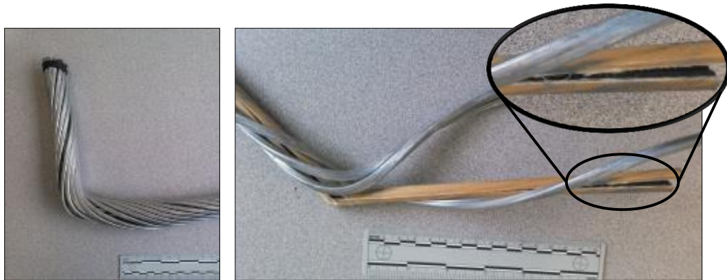
Figure 2: Laboratory induced damage through low-velocity impact. The composite core fails in shear resulting in a long crack extending into the conductor. Photo courtesy of Daniel Waters.
