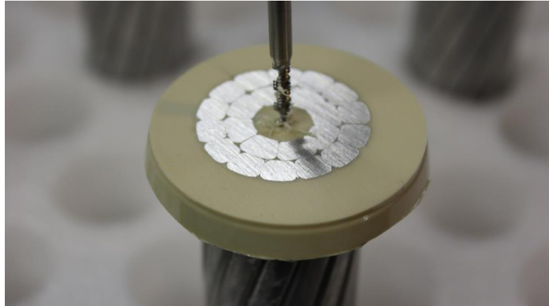
Figure 56: Holes are drilled and tapped.
