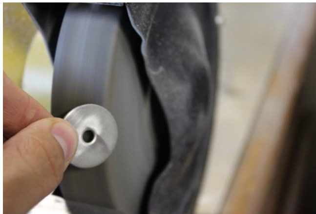
Figure 51: Cleaning of hardware using a polishing wheel.
