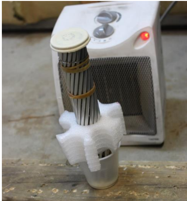
Figure 42: The conductor ends are potted in fast-curing epoxy.
