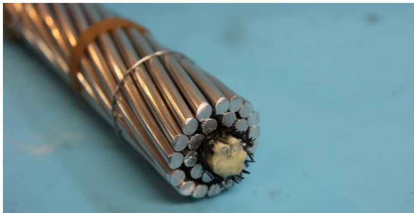
Figure 41: The re-assembled conductor sample with the steel core off-set.
