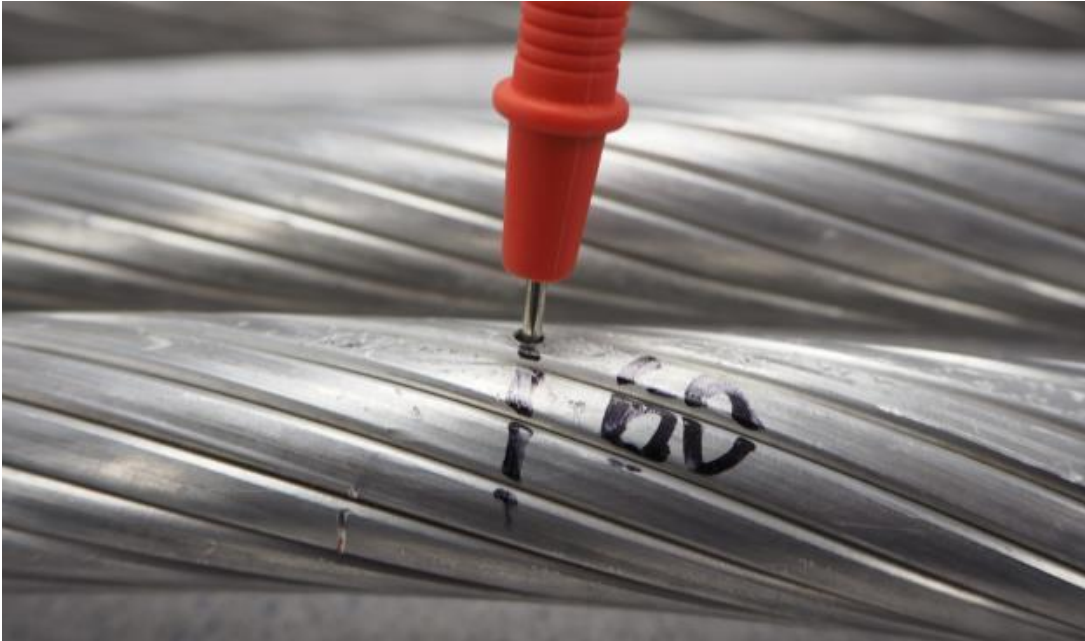
Figure 172: Metal probe inserted to make electrical contact between the Al and the CFRP.
