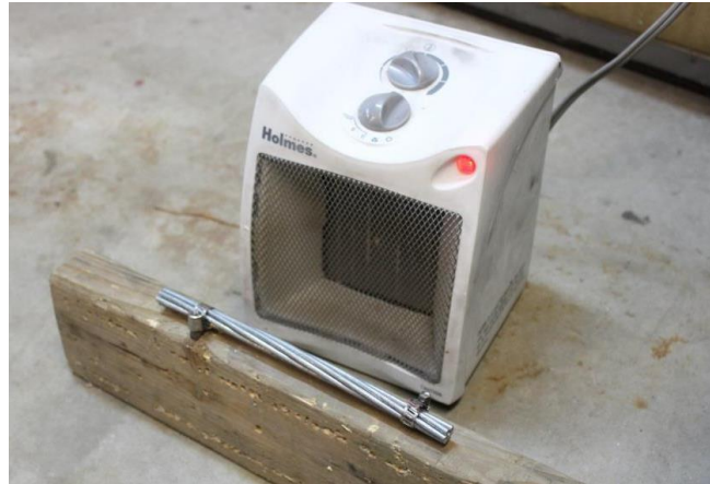
Figure 38: Pre-heating the core.
