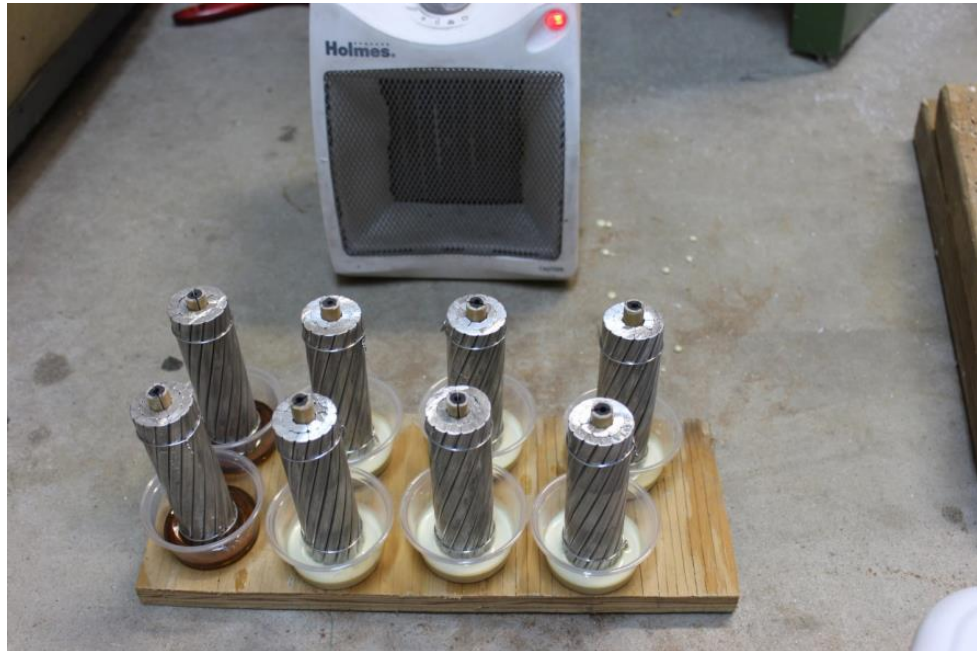
Figure 54: The conductor ends are potted in fast-curing epoxy. The uncured epoxy is a brown translucent liquid, while the cured epoxy is opaque beige.
