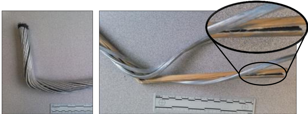
Figure 2 (repeated): Laboratory induced damage through low-velocity impact. The composite core fails in shear resulting in a long crack extending into the conductor. Photo courtesy of Daniel Waters.
