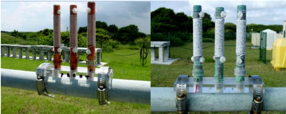
Figure 34: Wire-on-bolt test ASTM G116-99. Left) Immediately after installation at the Kennedy Space Center beach corrosion test site. Right) After 30 days. Source: (CorrosionDoctors 2014)
