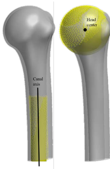
Figure 3. Best-fitting cylinder for the metaphyseal cylinder (left) and the best-fitting sphere for the humeral head (right). The nodes on the cortical shell used to find the best-fitting geometries are represented as yellow scatter points; the analytical surfaces are represented in shaded yellow.
