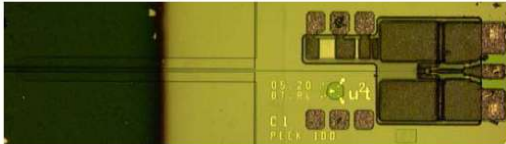
Fig. 2.16 photodiode chip featuring a passive optical waveguide, an integrated bias network and an LC circuit, creating an inductive peaking at 100GHz (Stohr, et al. 2007).
