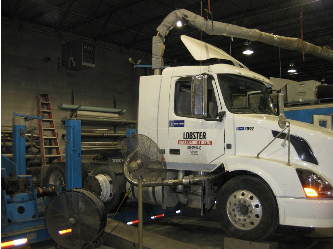
Figure 39: '08 Volvo day cab on dynamometer with insulated pipe leading to ETaPS and CVS dilution tunnel.
