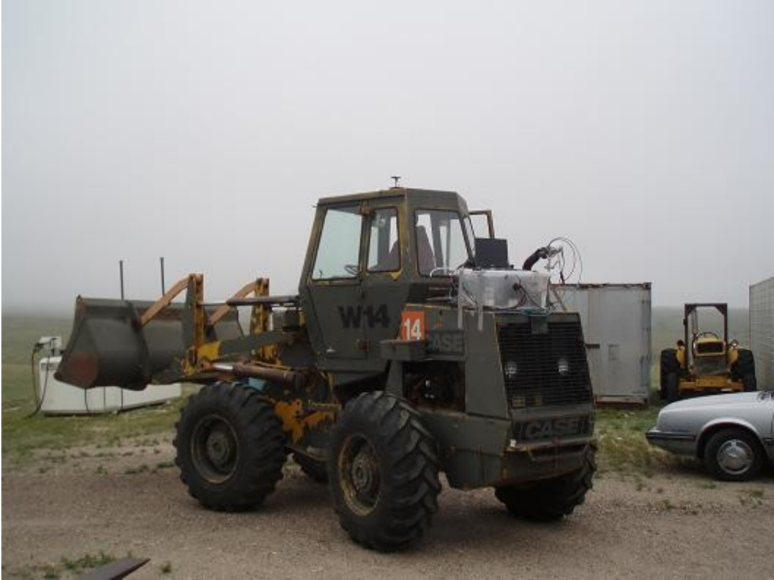
Figure 29: ETaPS mounted on a diesel Caterpillar front loader. As in all installations power was provided from an on-board 110V generator grounded to the vehicle
