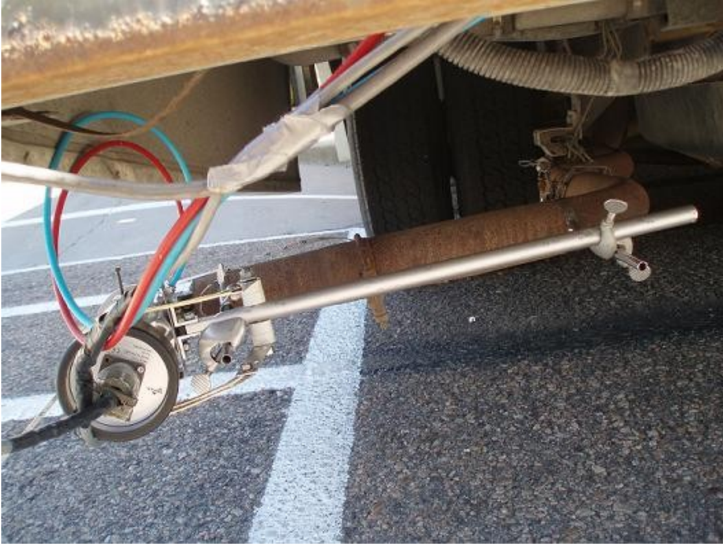
Figure 31: ETaPS mounted analyze the particles exiting the exhaust of a gasoline powerd 1996 Winnebago Itasca motor home powered by a GM 454 cu.in. V8 engine.
