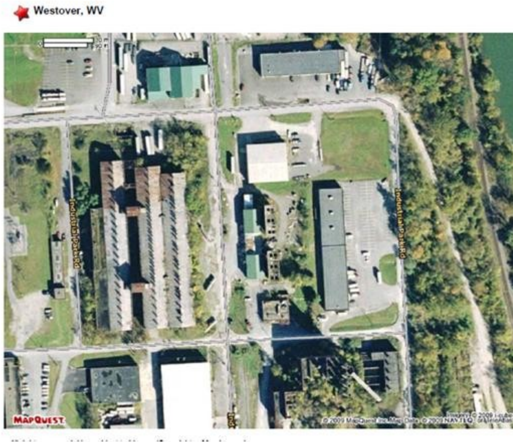
Figure 34: Satellite photo of Westover WVU facility and surroundings. The building at the top right, with visible trucks parked on the east side, is the dynamometer facility. The RSD scaffolding and measurement system were set up at the black dot located at in the center south end of the parking lot of the testing facility. RSD measurements were taken across industrial park road. All readings were taken with truck traveling on an uphill slope westbound. Frequently the repeat measurements were made by looping around the small rectangle of roadways starting with a left turn down the center of the picture.
