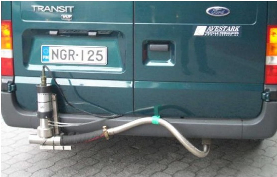
Figure 36: Dekati's experimental setup for measuring on-road vehicle emissions.
