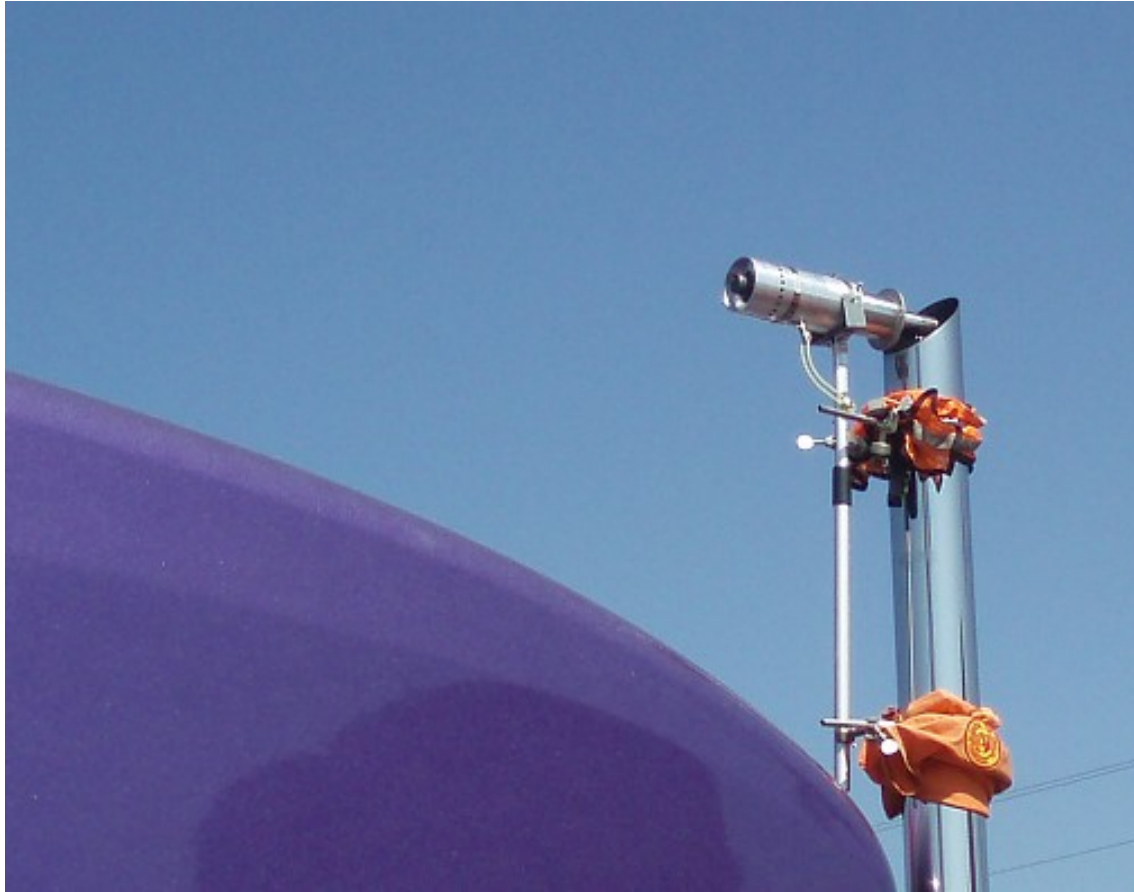
Figure 28: ETaPS on a 7” exhaust stack from a DPF equipped 2006 MY Peterbilt tractor.
