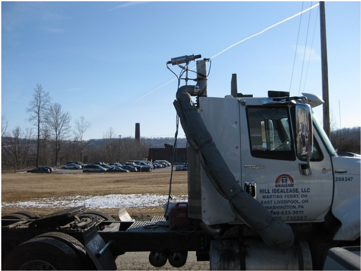
Figure 37: ETaPS mounted on left side of elevated exhaust pipe. O 2 sensor mounted on right side of elevated exhaust. Data acquisition equipment, air pump, and generator are visible on the metal platform behind the cabin. Of note is the overhead power line on the upper right later shown to cause interference with the ETaPS signal.
