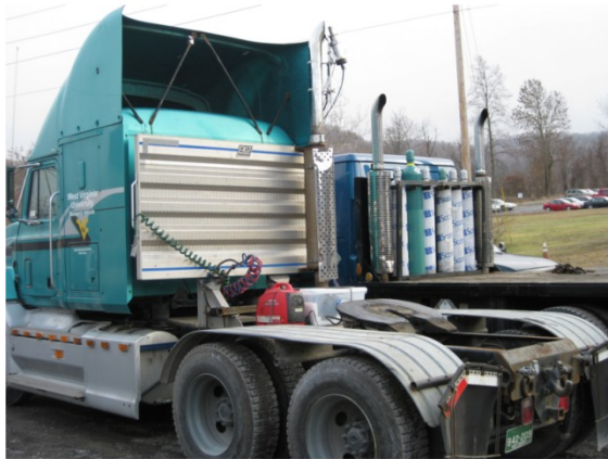
Figure 38: Three angles of an ETaPS mounting. ETaPS and O 2 sensor are attached to the exhaust pipe. Data acquisition equipment, air pump, and generator are secured to metal platform behind the cabin.
