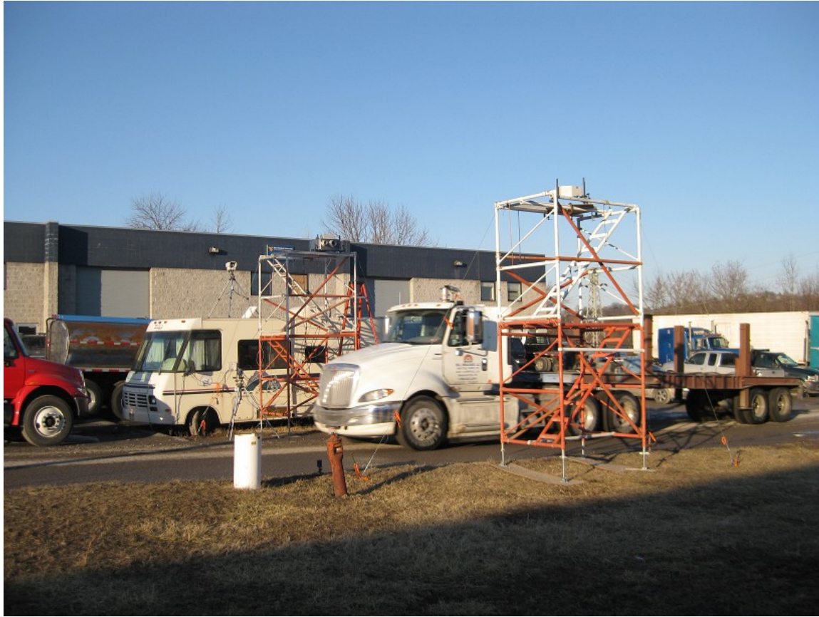
Figure 35: RSD setup outside WVU testing facility. To the rear of the rear scaffolding is the Mobile laboratory (Itasca) which housed the computer for the RSD.
