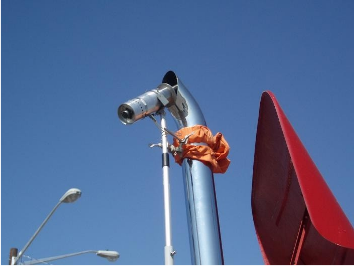
Figure 27: ETaPS mounted on the 5" tailpipe of a 2000 MY Peterbilt tractor. The cloth was used to protect the vehicle (for sale in a dealer lot) from scratches.
