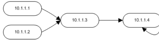
Figure 1.3: Intrusion detection alarms from Table 1.1 as a directed graph
