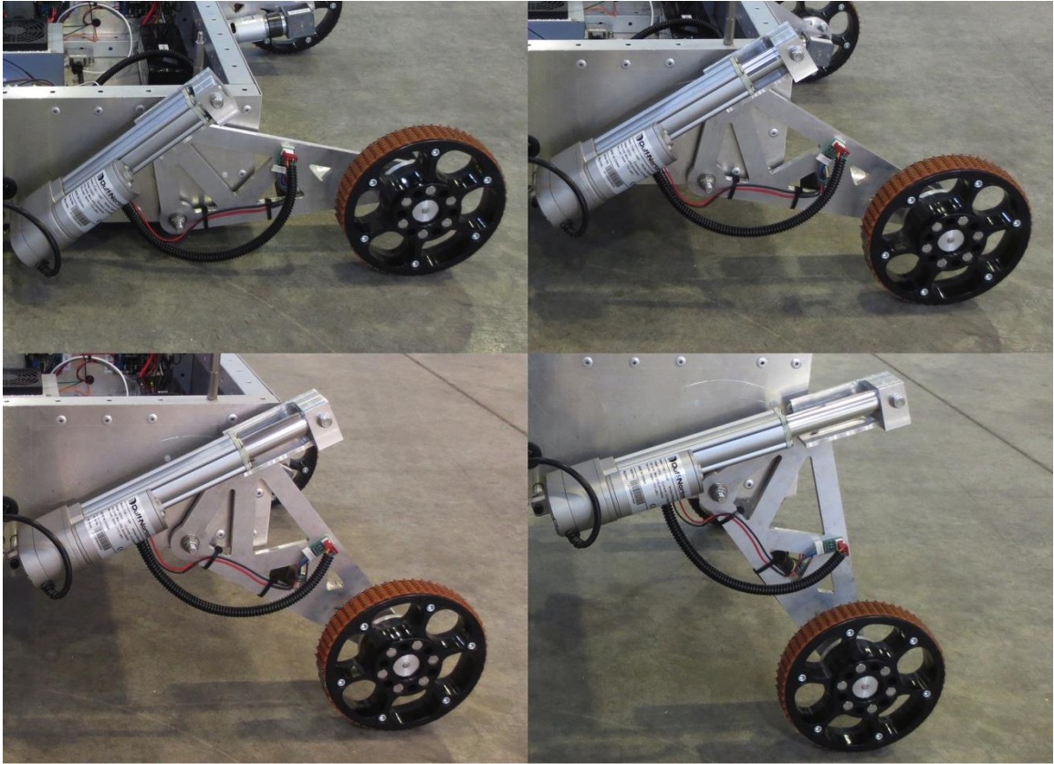
Fig. 4. Self-leveling mechanism of the landing platform.
