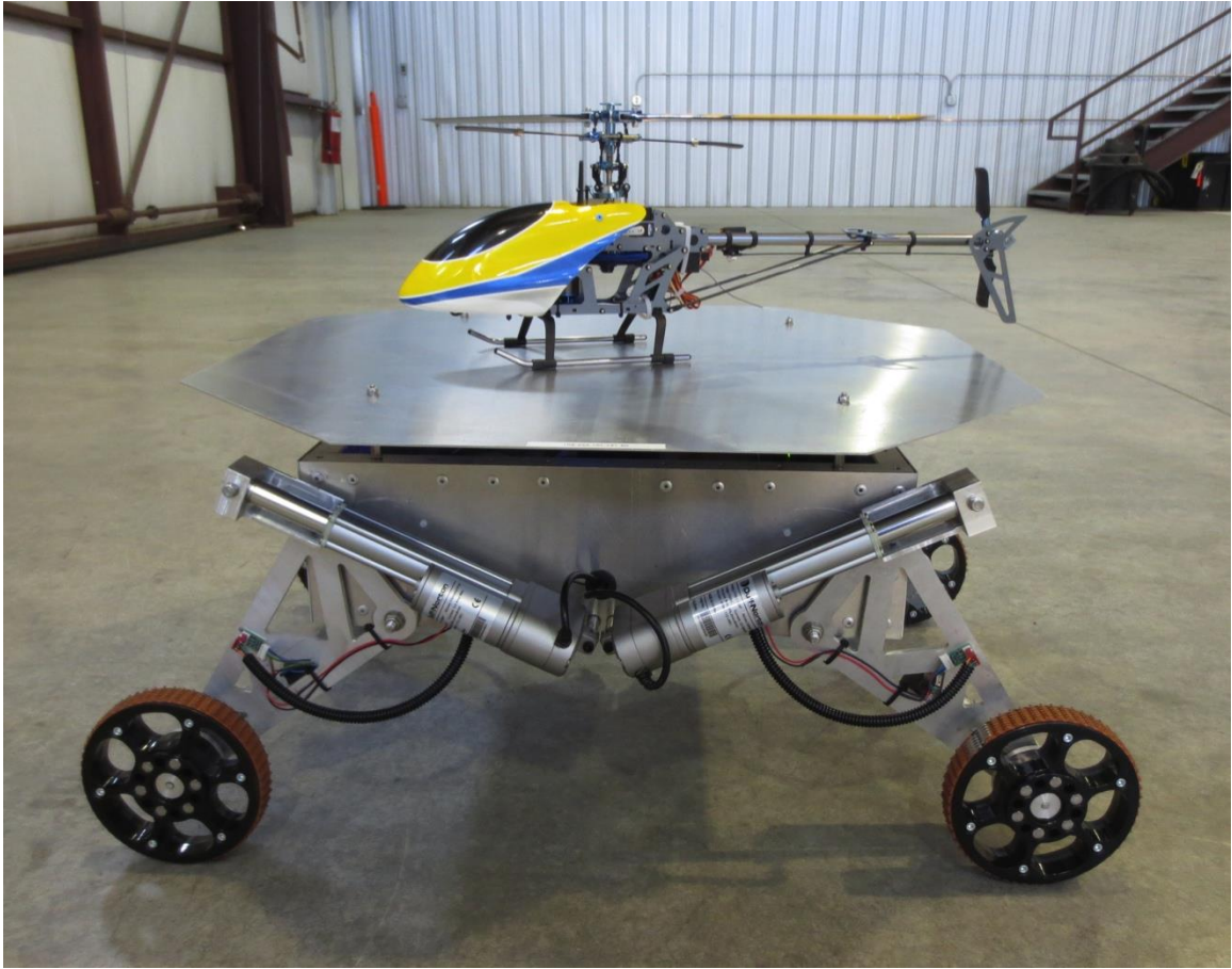
Fig. 5. Landing platform prototype with TREX 450 helicopter on board.
