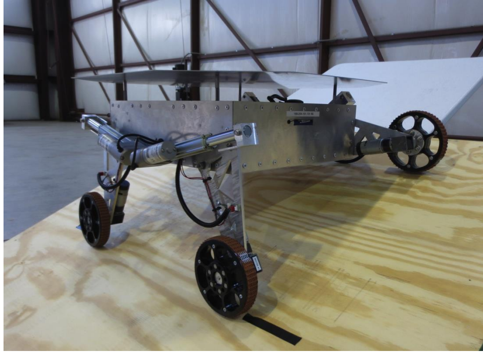
Fig. 35. Photograph of the transverse X-axis self-leveling test.
