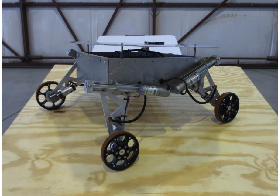
Fig. 39. Photograph of combined self-leveling test.
