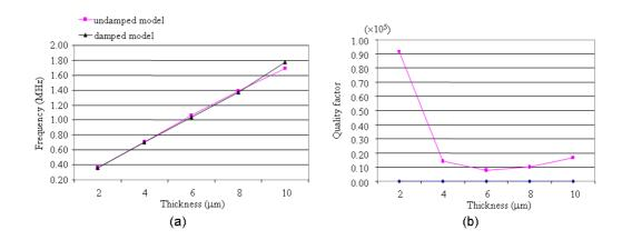
Figure 14: Frequency (a) and quality factor (b) as functions of the mirror size in model D.
