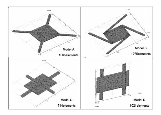
In all the four models, the peripheral beams connected to the central mirror are assumed fixed at the end; the mirror in the middle is free to vibrate. Both the beams and the mirror have the same thickness. The entire device is considered to be thermally insulated and the initial temperature is set to 300K.
