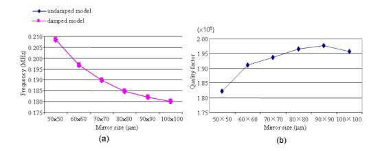
Figure 9: Frequency (a) and quality factor (b) as functions of the beam width in model A.
