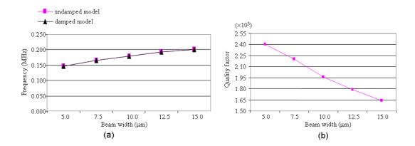
Figure 10: Frequency (a) and quality factor (b) as functions of the mirror size in model B.
