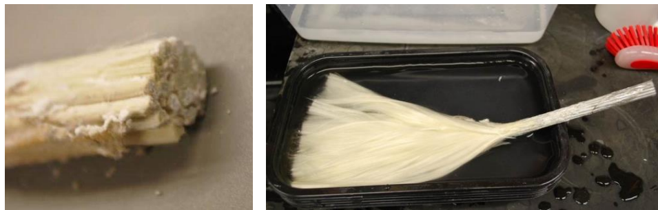
Figure 47: Damage to the ACCR core.
