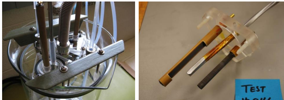
Figure 21: C 3 LARC sample holders. The sample holders are based on the KF-40 vacuum flange system which provides a standardized system for the easily modifiable sample holders.
