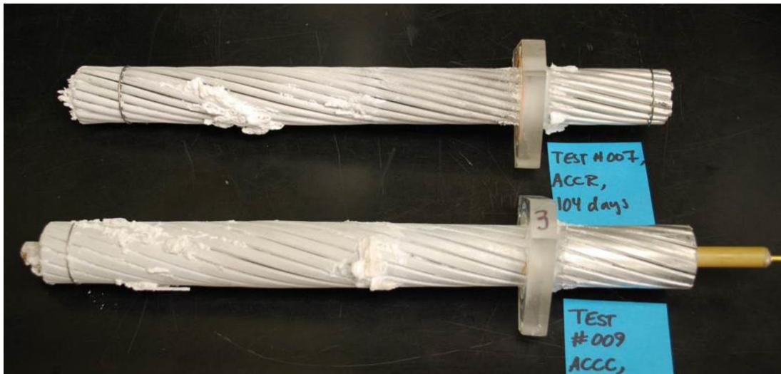
Figure 38: ACCR and ACCC after Test A. ACCR (top) and ACCC (bottom) had very little visual damage before cleaning.
