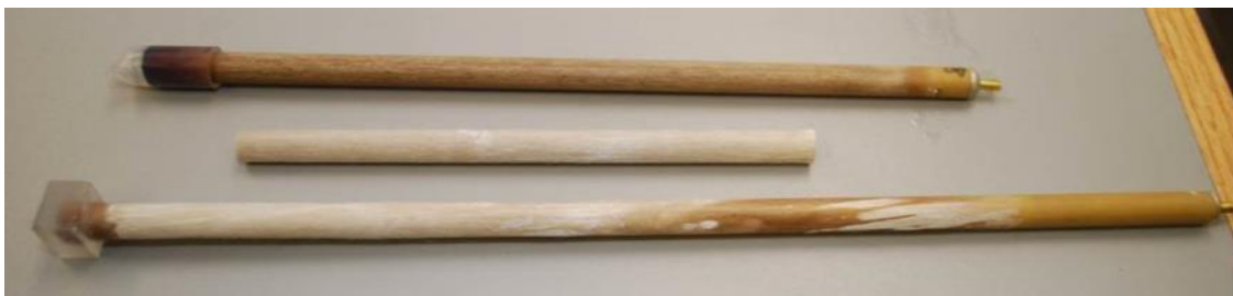
Figure 67: Three samples of ACCC core exposed to 85°C for approx. 100 days. Top: Sample exposed to same electrolyte as used in this study, but without presence of aluminum hydroxide. Middle: sample placed in the “slurry” of aluminum hydroxide at the bottom of the testing cell during Test A. Bottom: Sample from Test A.
