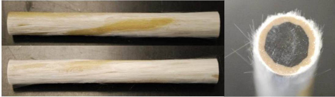
Figure 55: Three views of the same ACCC sample (Test B). The minor surface damage is similar to that seen in Test A.
