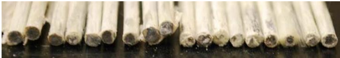
Figure 57: End view of the ACCR core strands (Test B).
