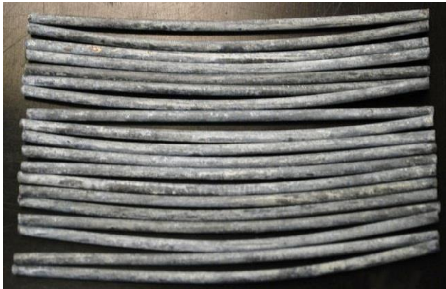
Figure 54: Neither the ACSS core had any signs of rust (Test B).
