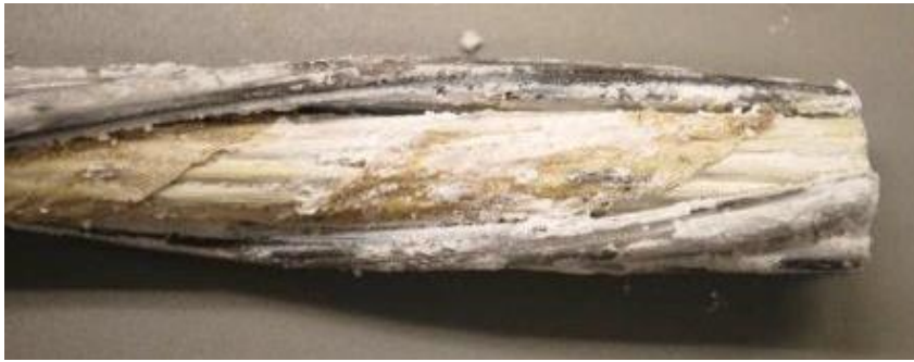
Figure 46: The metal-matrix composite core of ACCR after Test A, still surrounded with some of the aluminum strands.
