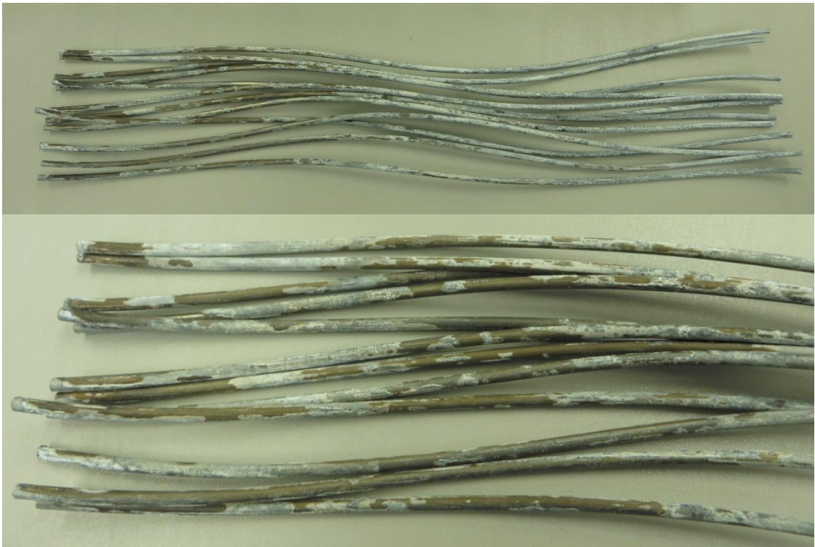
Figure 45: Core strands of ACSS after Test A. The coating is lost in areas above the liquid level.
