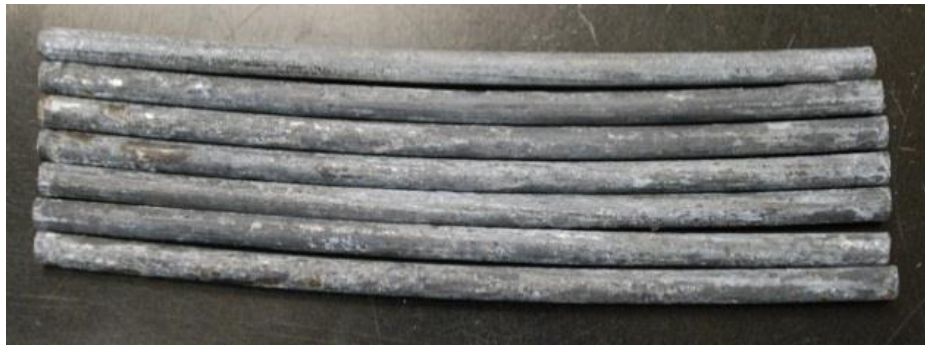
Figure 53: No signs of rust on the ACSR core (Test B).
