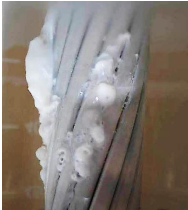
Figure 6: Formation of \text{Al}(\text{OH})_3 on the ACCC sample.
