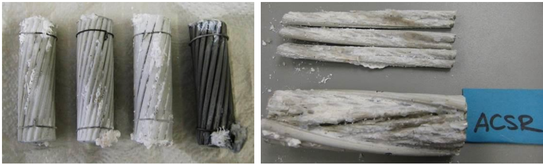
Figure 28: Samples from Test B. Samples just taken out from Test B (left), and typical sample before cleaning (right).
