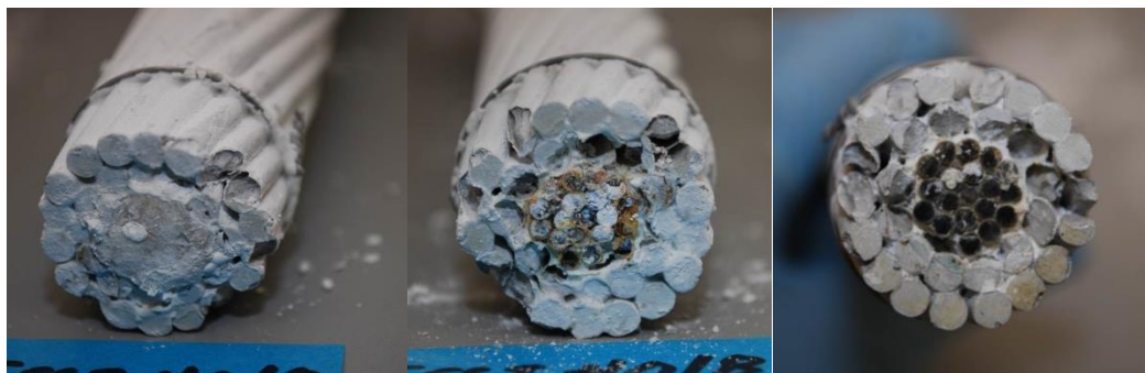
Figure 40: Localized corrosion at the end of the ACSS sample.
