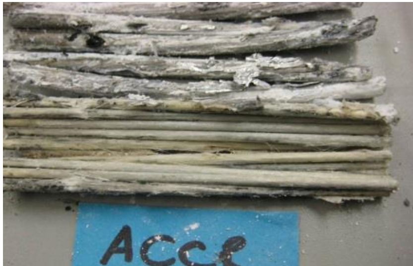
Figure 56: The ACCR sample before cleaning (Test B).
