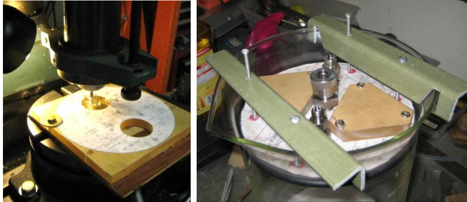
Figure 20: Manufacturing of the C 3 LARC testing cell. The C 3 LARC instrument can be built with simple manufacturing methods. Drawings are found in Appendix A.
