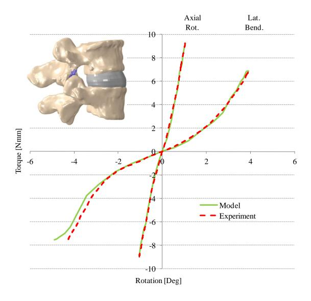
Figure 3.7 Comparison of model predicted and experimentally measured torque-rotation response of the L4-L5 FSU in axial rotation and lateral bending following resection of the supraspinous, interspinous, posterior longitudinal, anterior longitudinal, and intertransverse ligaments.
