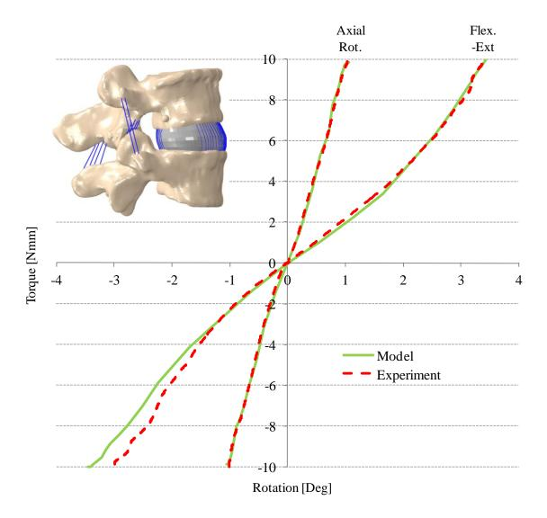
Figure 3.3 Comparison of model predicted and experimentally measured torque-rotation response of the L4-L5 FSU in flexion-extension and axial rotation following resection of the supraspinous ligament.
