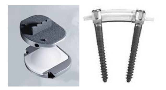
Figure 2.4 Ball on socket total disc replacement device with metallic endplates and polyethylene core (left) and dynamic posterior stabilization device with pedicle screws (right) (Murtagh *et al.*, 2011, us.synthesprodisc.com, 2011).
