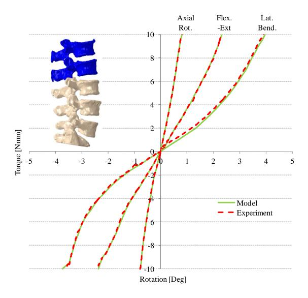
Figure 4.2 Comparison of model predicted and experimentally measured torque-rotation response of the intact L1-S1 multi-segment spine at level L1-L2 in flexion-extension, lateral bending, and axial rotation.
