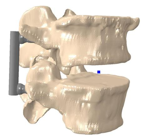
Figure 5.1 L4-L5 FSU instrumented with posterior stabilization device. Screws inserted through the pedicles. Rods modeled as titanium.
