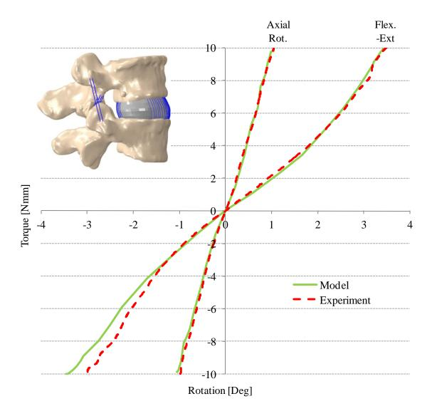
Figure 3.4 Comparison of model predicted and experimentally measured torque-rotation response of the L4-L5 FSU in flexion-extension and axial rotation following resection of the supraspinous and interspinous ligaments.
