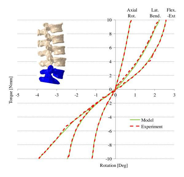
Figure 4.6 Comparison of model predicted and experimentally measured torque-rotation response of the intact L1-S1 multi-segment spine at level L5-S1 in flexion-extension, lateral bending, and axial rotation.
