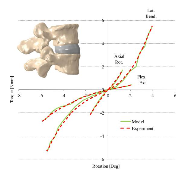
Figure 3.9 Comparison of model predicted and experimentally measured torque-rotation response of the L4-L5 FSU in flexion-extension, axial rotation and lateral bending following resection of the supraspinous, interspinous, posterior longitudinal, anterior longitudinal, intertransverse, and facet capsular ligaments, as well as the facet joints.
