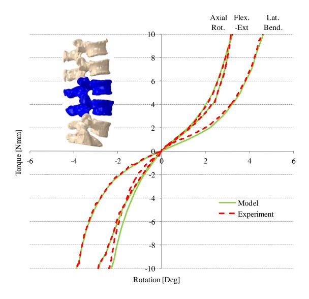
Figure 4.4 Comparison of model predicted and experimentally measured torque-rotation response of the intact L1-S1 multi-segment spine at level L3-L4 in flexion-extension, lateral bending, and axial rotation.
