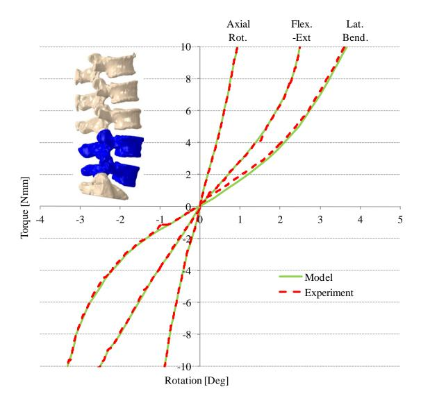
Figure 4.5 Comparison of model predicted and experimentally measured torque-rotation response of the intact L1-S1 multi-segment spine at level L4-L5 in flexion-extension, lateral bending, and axial rotation.
