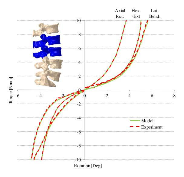
Figure 4.3 Comparison of model predicted and experimentally measured torque-rotation response of the intact L1-S1 multi-segment spine at level L2-L3 in flexion-extension, lateral bending, and axial rotation.
