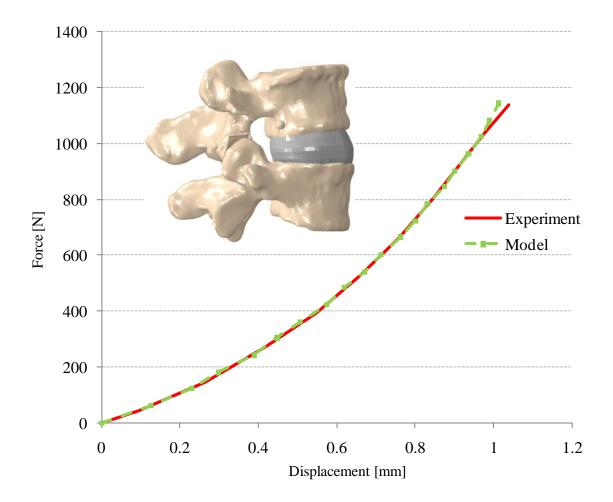
Figure 3.10 Comparison of model predicted and experimentally measured forcedisplacement response of the L4-L5 FSU in axial compression following resection of the supraspinous, interspinous, posterior longitudinal, anterior longitudinal, intertransverse, and facet capsular ligaments, as well as the facet joints.
