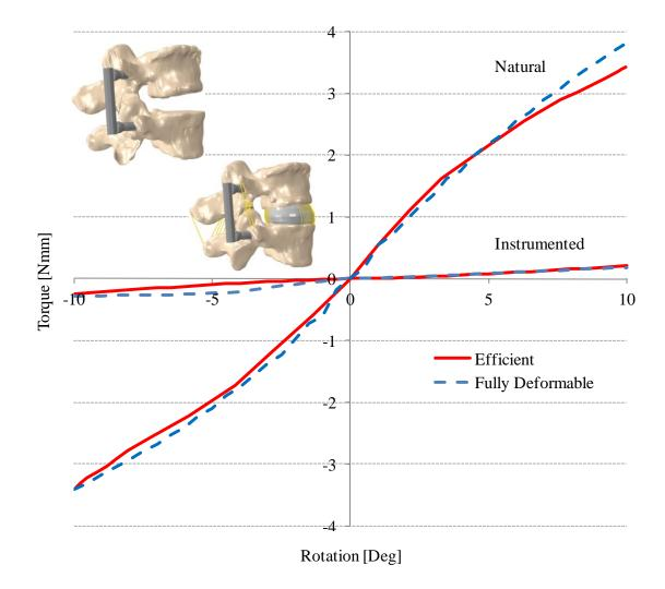
Figure 5.2 Comparison of torque-rotation behavior for intact FSU and FSUs instrumented with titanium and PEEK posterior fusion rods.
