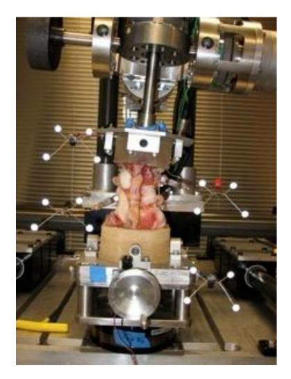
Figure 2.5 University of Washington Applied Biomechanics Lab Multi-Axis Spine Simulator.
