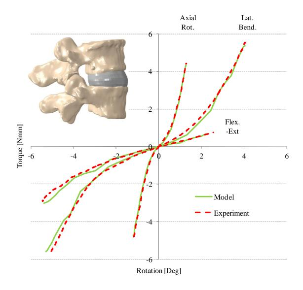
Figure 3.8 Comparison of model predicted and experimentally measured torque-rotation response of the L4-L5 FSU in flexion-extension, axial rotation and lateral bending following resection of the supraspinous, interspinous, posterior longitudinal, anterior longitudinal, intertransverse, and facet capsular ligaments.
