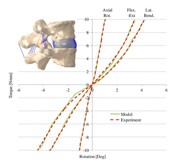
Figure 3.2 Comparison of model predicted and experimentally measured torque-rotation response of the intact L4-L5 FSU in flexion-extension, lateral bending, and axial rotation.
