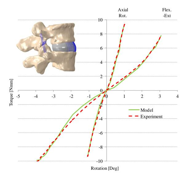
Figure 3.5 Comparison of model predicted and experimentally measured torque-rotation response of the L4-L5 FSU in flexion-extension and axial rotation following resection of the supraspinous, interspinous, and posterior longitudinal ligaments.
