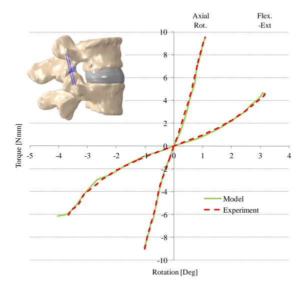
Figure 3.6 Comparison of model predicted and experimentally measured torque-rotation response of the L4-L5 FSU in flexion-extension and axial rotation following resection of the supraspinous, interspinous, posterior longitudinal, and anterior longitudinal ligaments.
