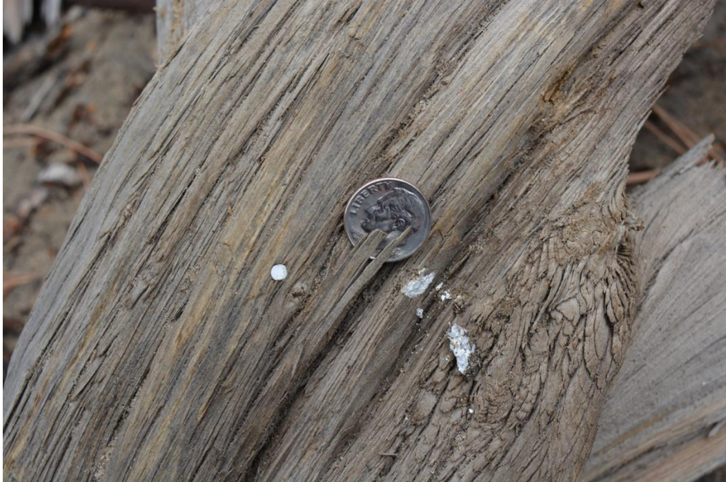
White nail head as ground control point. Dime for scale.
