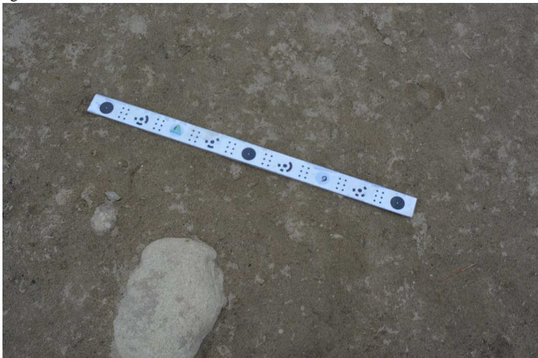
Scale bar. Approximately 1.2 meters across. The four circular patterns are the unique coded markers.
