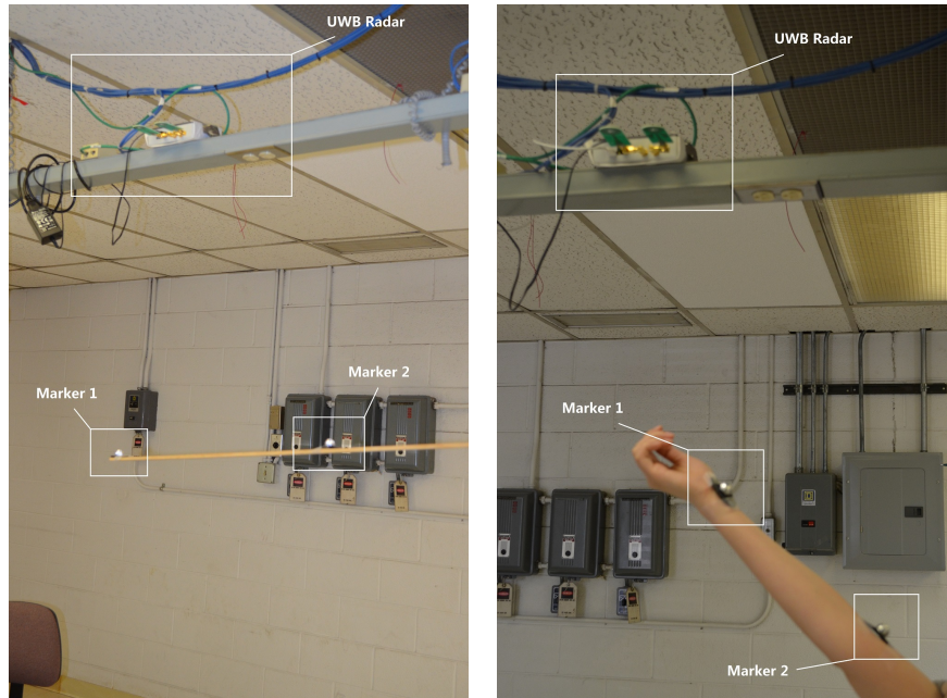
Figure 2.12: Scenarios for Experiment I with a moving ruler (left), and Experiment II with a moving arm (right).
