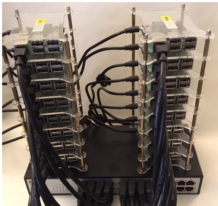
Figure 17. Parallel iterative instrumentation setup with a cluster of Raspberry Pi 3
