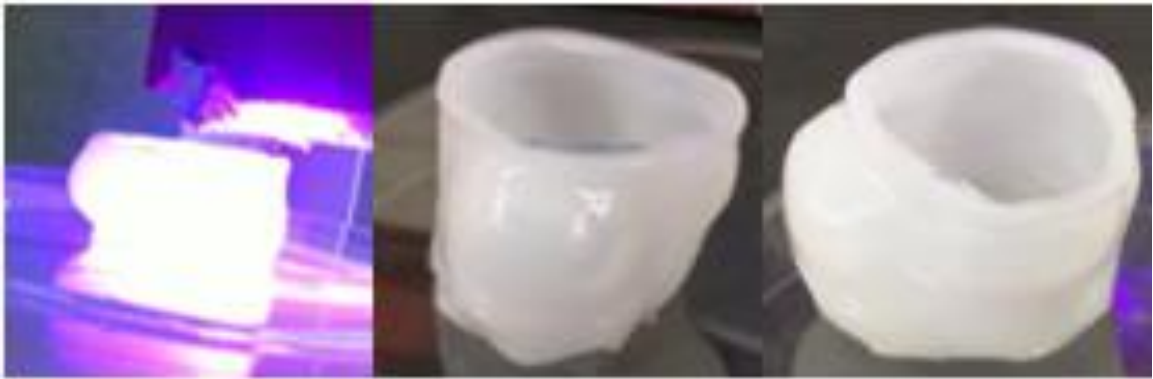
Figure 66. Aortic scaffold being printed under 365 nm UV light with intensity of 410 mW/cm 2 ; finished scaffold from two angles, 15 % PEGDA 2% HPMC w/v.
