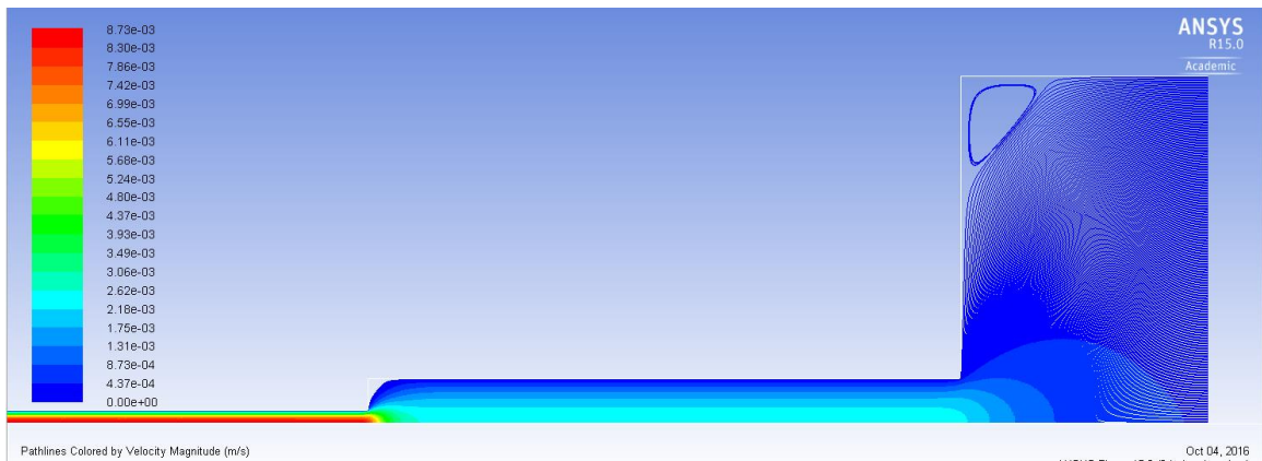
Figure 56. The pathlines colored by velocity magnitude.
