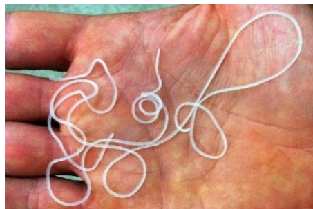
Figure 72. The extrusion can be configured such that the material crosslinks before contacting the print bed and thus creates a long elastic thread.
