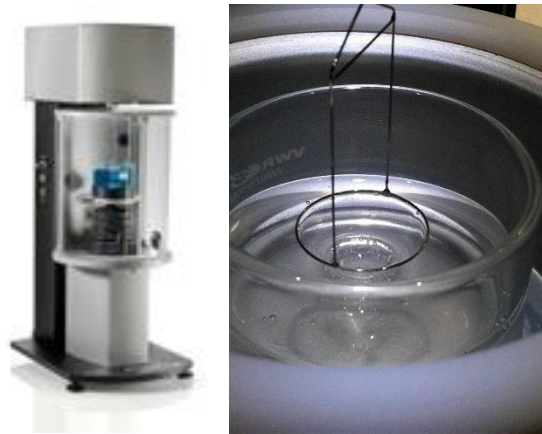
Figure 34. Picture of whole apparatus and close up of the platinum du Nouy ring.
