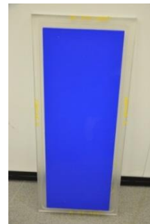
Standard Testing plate: Length=600mm Width=218mm
