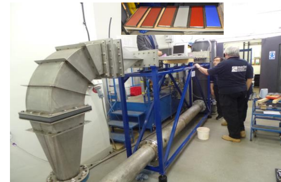
Turbulent channel set-up for “Roughness Function” measurement
