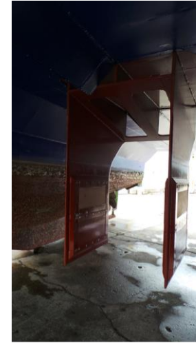
The Moon pool strut in place
