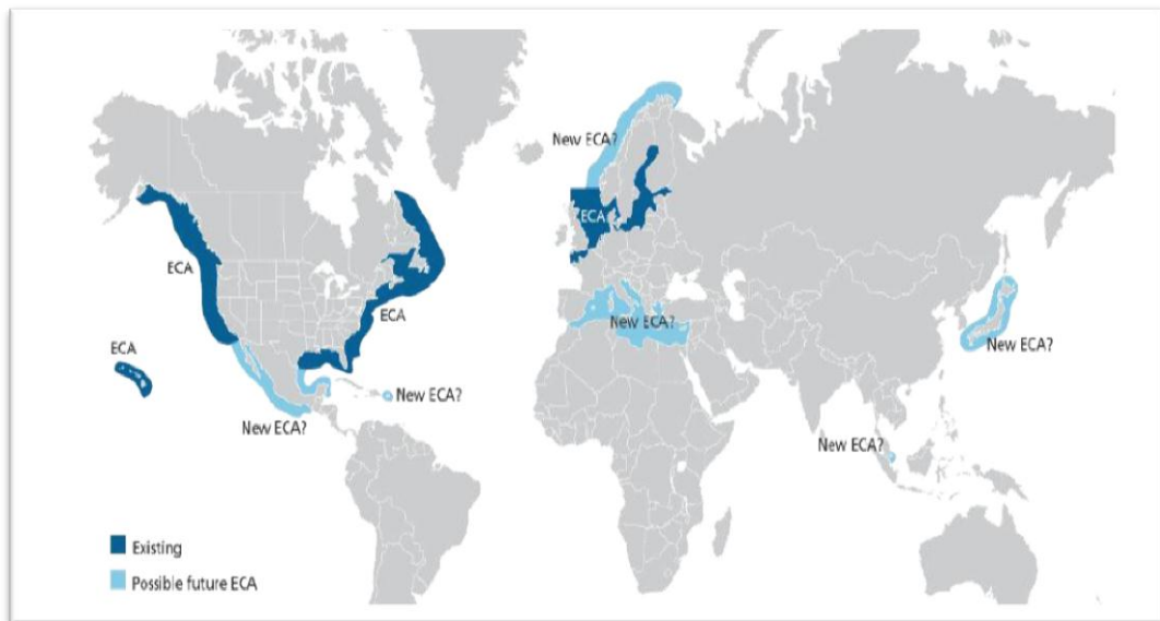
Figure 2.13: Existing and potential new ECAs (Source: SSP, 2012)
