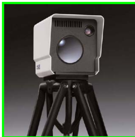
Figure35: Thermalvision camera for port and channel security.
