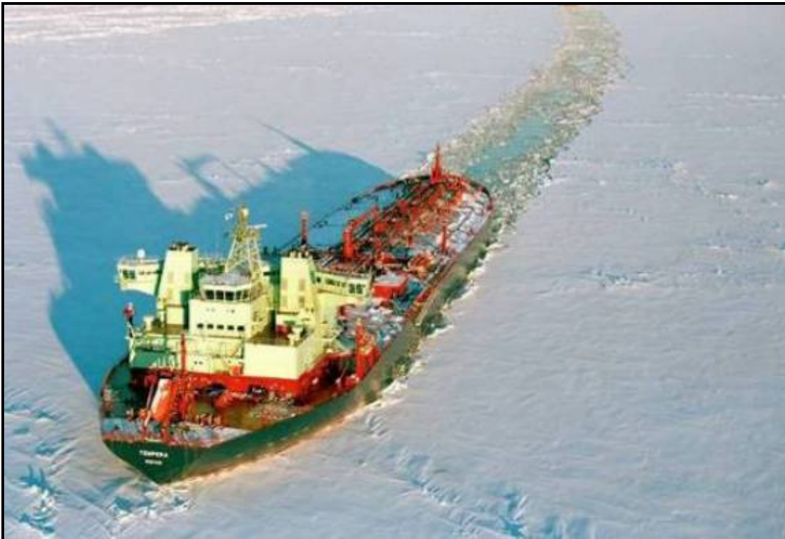
Figure 2-4: A DAS Tanker Ship Breaking the Ice while Steering Astern. Source: (Wilkman, n.d.)
