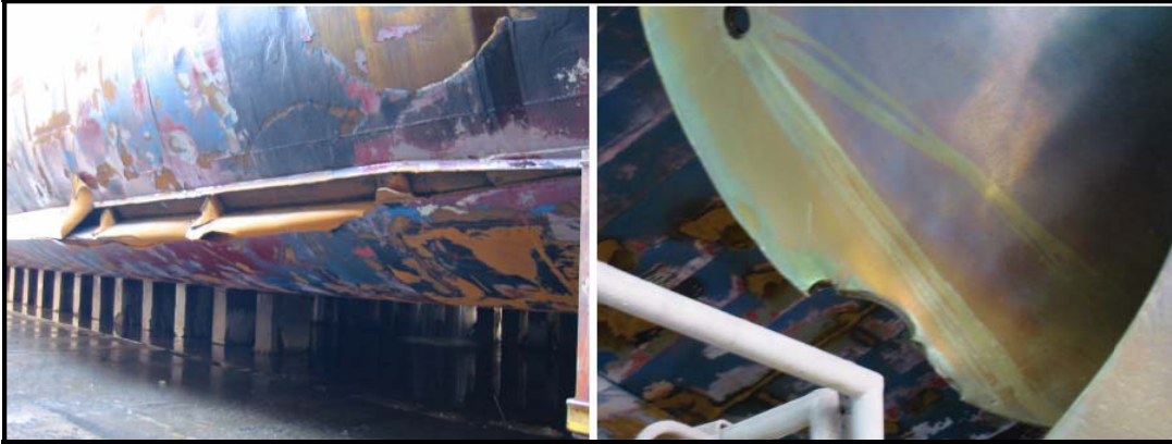
Figure 3-2: A Bilge Keel Rupture and Propeller Damage of Ship Number 100. Source: (Hänninen, 2003)
