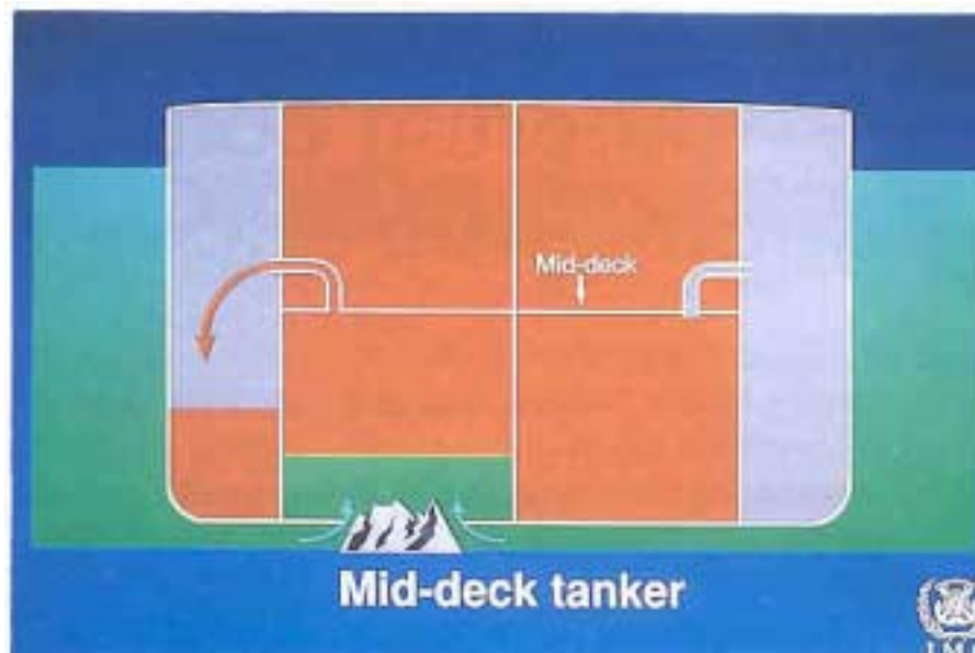
Fig. 33. General tank layout of a mid-deck tanker
