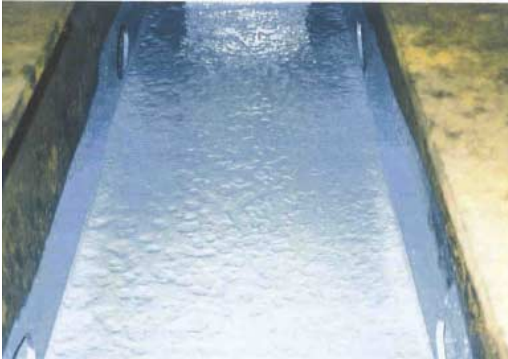
Fig. 22. Coating is the best solution when pitting occurs (Source: DNV paper series No.2000-P008. p.21)
