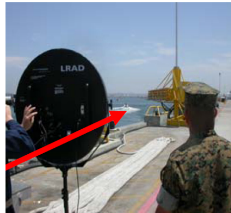
Figure 26: Small boat L-RAD test with USS Coronado's crew, distance of the small boat, 450 yards, receiving instructions loud and clear. Source: American Technology Corporation
