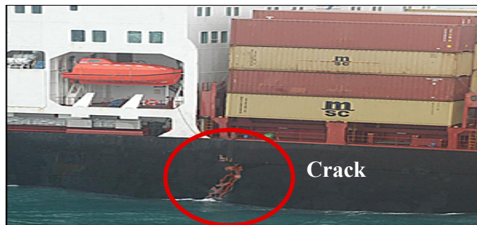
Figure 4.1 Large cracks in the ship's stern of MSC NAPOLI.
