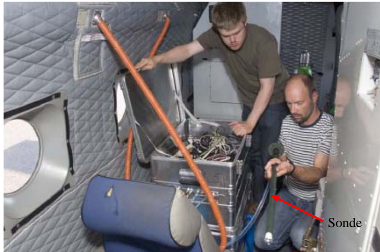
Figure 4-10. The scientist of Chalmers installing the sonde in the airplane
