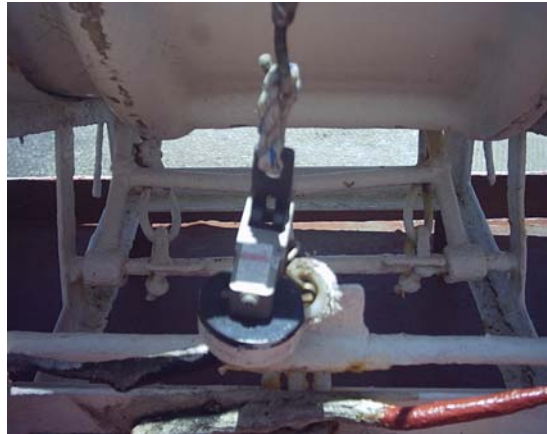
Painter not connected to the HRU.
