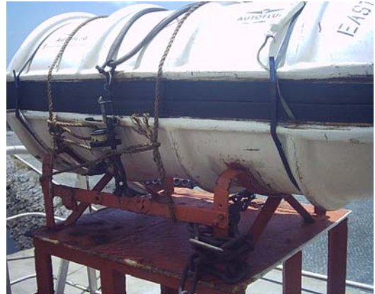
Painter not connected to the HRU.
