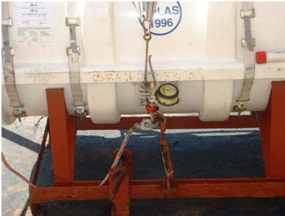
Painter incorrectly connected.
