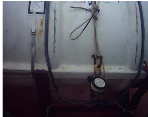
Free-flotation hampered by nylon rope.
