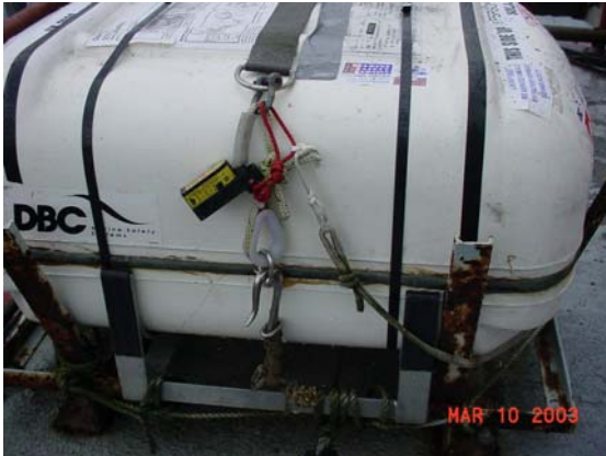
Painter and hook incorrectly connected.
