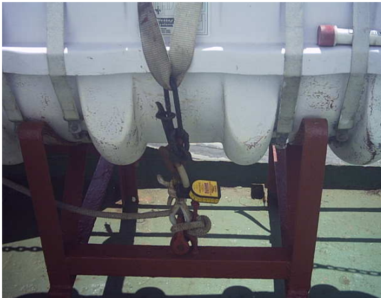
Painter connected to a fixed eye.
