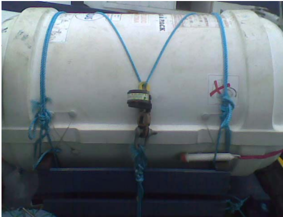
Painter not connected to weak link.
