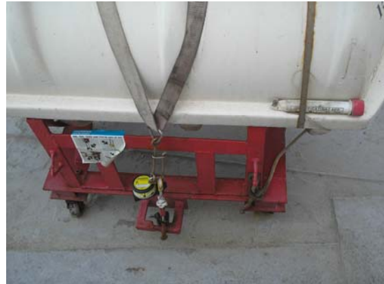
Figure 3.7 - HRU incorrectly installed. Figure 3.8 - HRU incorrectly installed.
