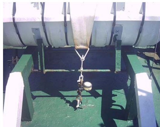
Painter not connected to the HRU.
