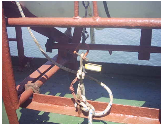
Painter connected directly to weak link.
