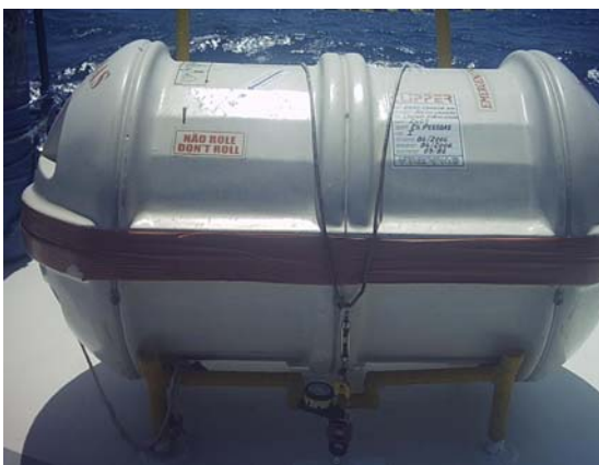
Painter not connected to the weak link.
