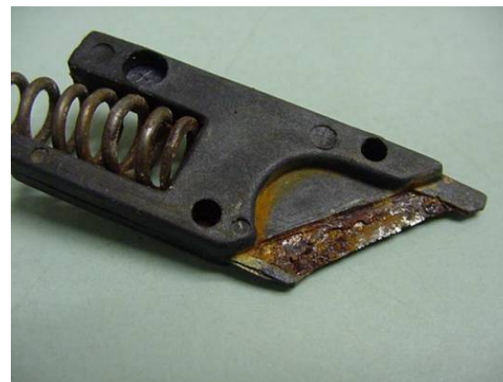
Figure 1.5 - Rusty blade. Source: AMSA.
