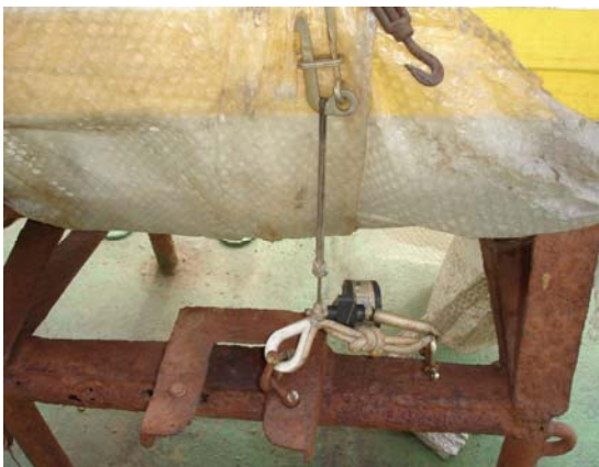
Painter and hook incorrectly connected.
