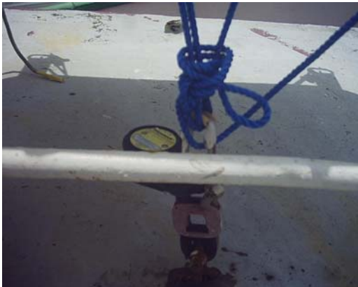
Painter not connected to the weak link.
