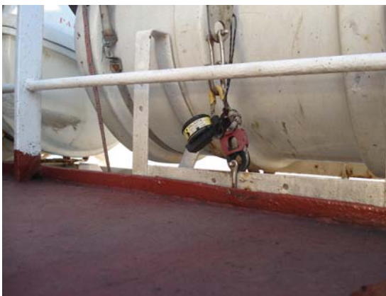
Painter not connected to the weak link.
