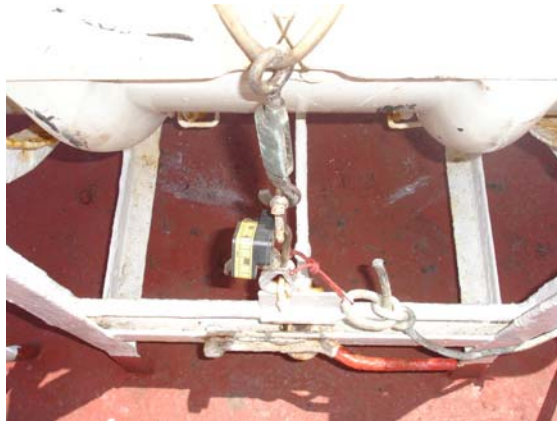
Painter incorrectly connected.
