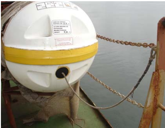
Painter connected to a fix point.
