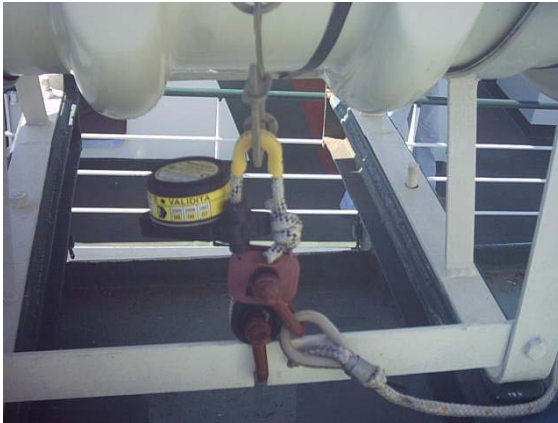
Expiry date missing.
