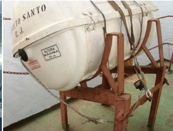
Painter incorrectly connected.
