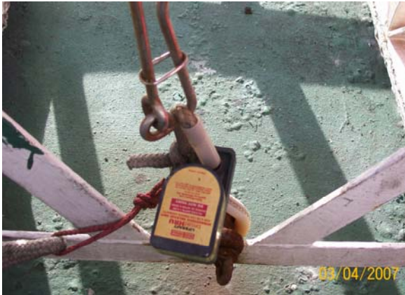
Painter connected directly to the weak link.
