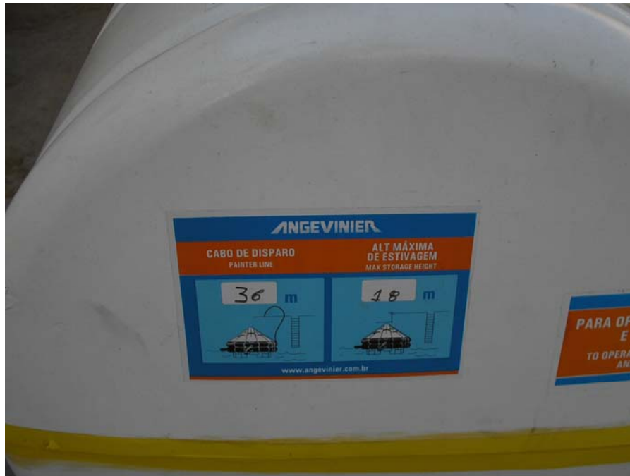
Figure 4.4 – Painter length incompatible with stowage height (actually 10 m) 22 .
