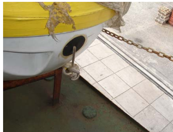
Painter not connected to the HRU.
