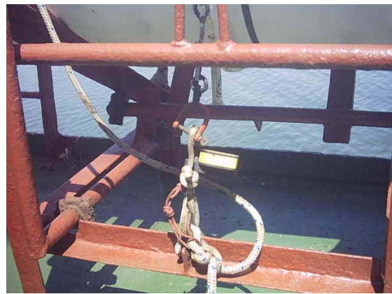
Painter incorrectly installed.
