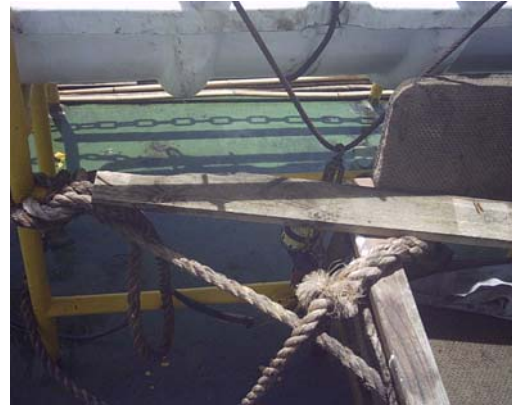
Figure 3.11 - Liferaft not ready for use.
