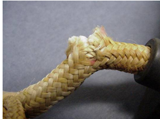
Figure 1.7 - Detail of incomplete cut. Source: AMSA.
