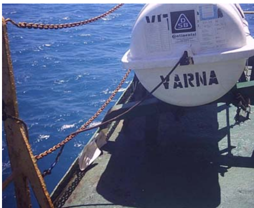
Painter connected to a fix point.
