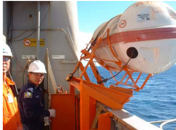
Painter connected to the cradle.
