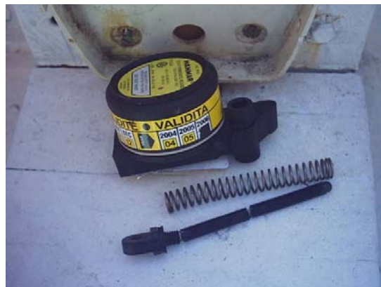
Figure 3.6 - Damaged bolt for EPIRB.
