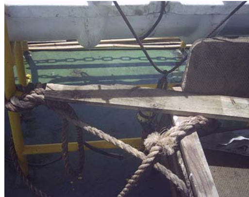
Manual launching obstructed.
