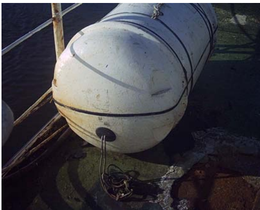
Internal weak link instructions missing.
