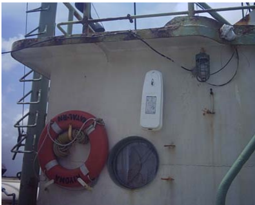
Obstruction to free-flotation.
