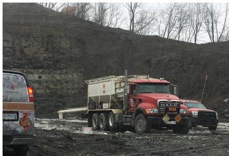
The truck in the center is loading ANFO into drill holes in preparation for rock blasting
