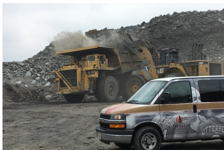
Students observe blasted overburden being loaded to move it from the working face
