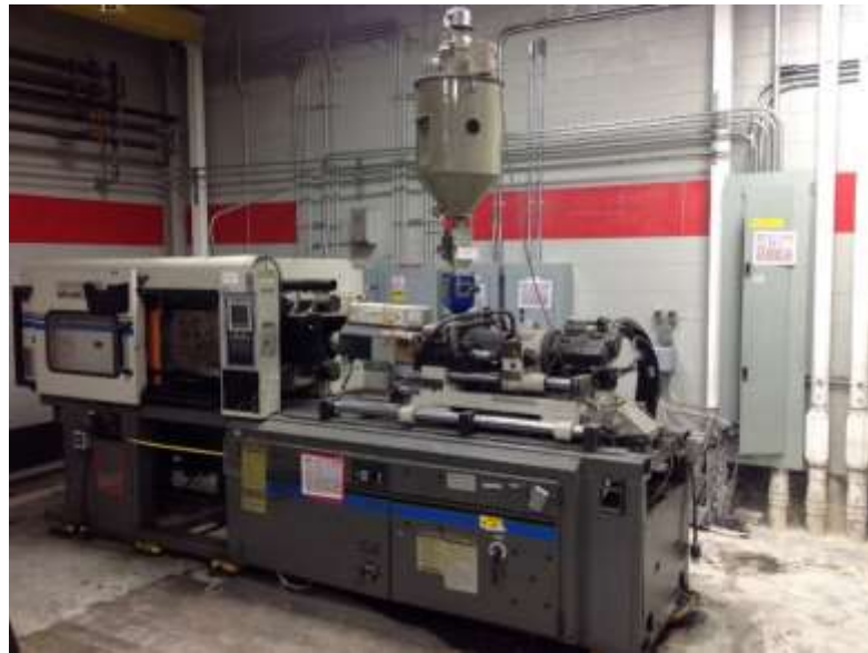
Figure H. 4 Injection molding press for experimental trials: Cincinnati Milacron (CML) VT-110
