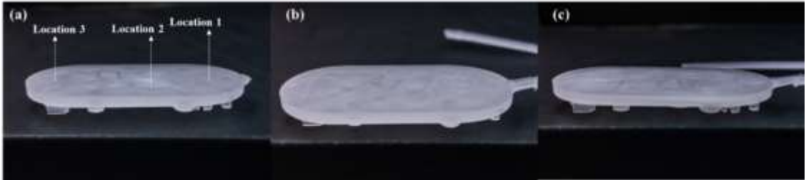
Figure 2.16 Injection molded parts using the machined mold with 3 mm mold depth (side-view): (a) 0 wt. % BA, (b) 1 wt. % BA, (c) 2 wt. % BA
