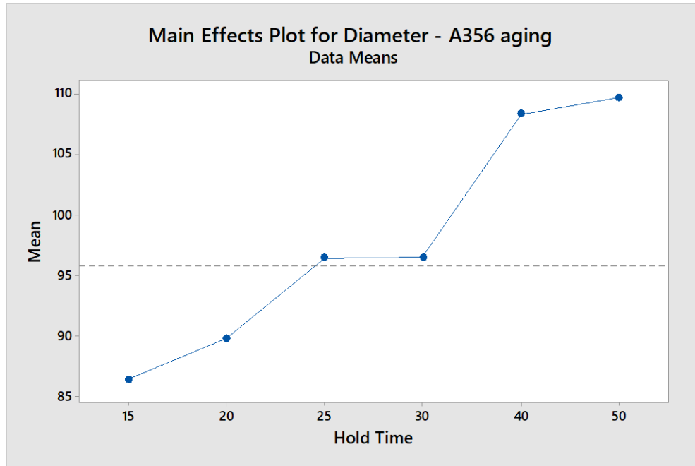
Figure 117 - Main effects plot for grain size - A356 aging
