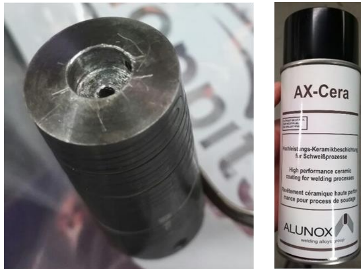
Figure 94 - left) Nozzle without tip right) Boron Nitride ceramic spray
