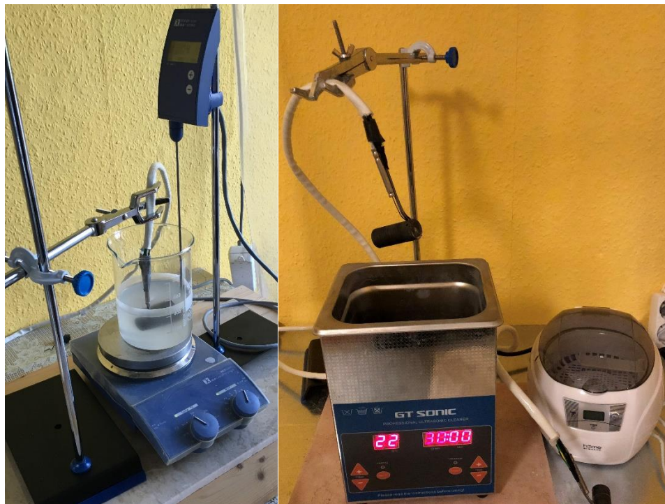
Figure 123 - Nozzle cleaning left) magnetic mixer right) ultra-sonic
