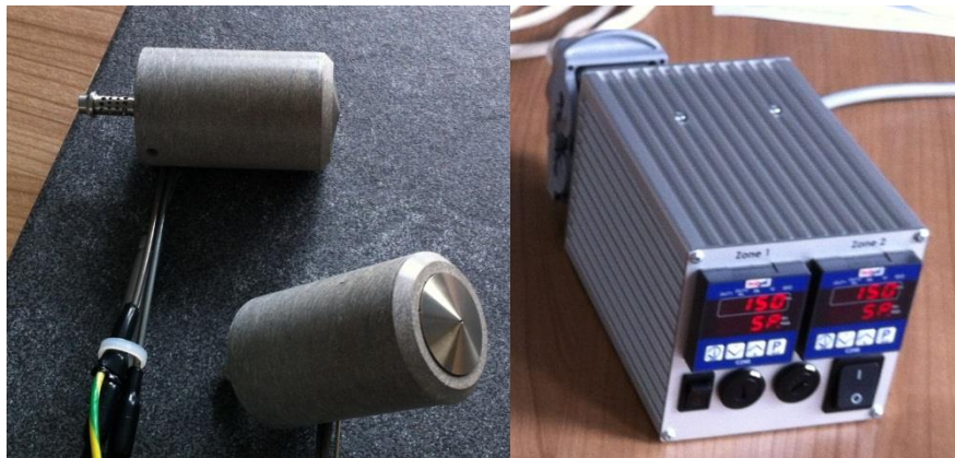
Figure 66 – Resistive heating channel and control unit
