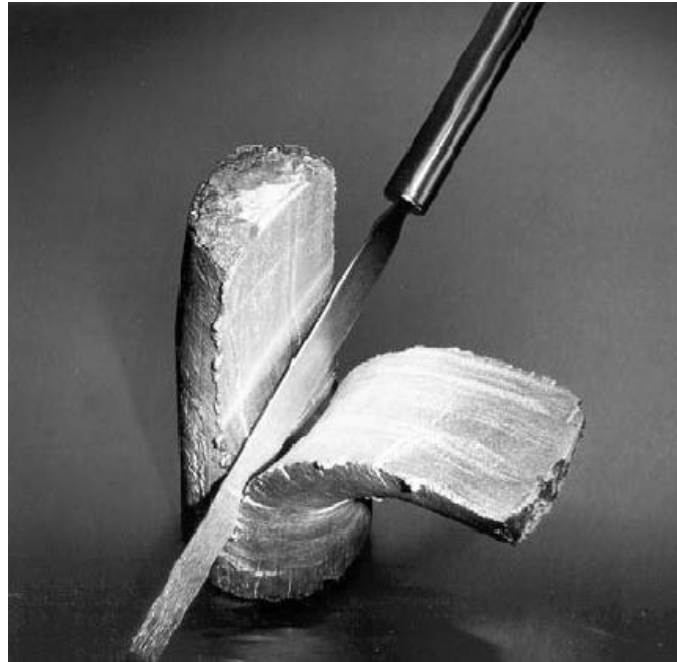
Figure 5 - Aluminum alloy billet at f_s=0.5 exhibits a consistency of modeling clay [13]
