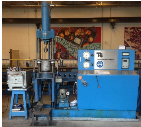
Figure 71 - 0.5MN extrusion press and recorded processing parameter
