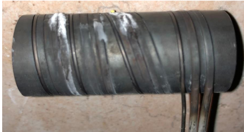
Figure 83 - Nozzle inside with resistive coil heaters and thermocouple connection
