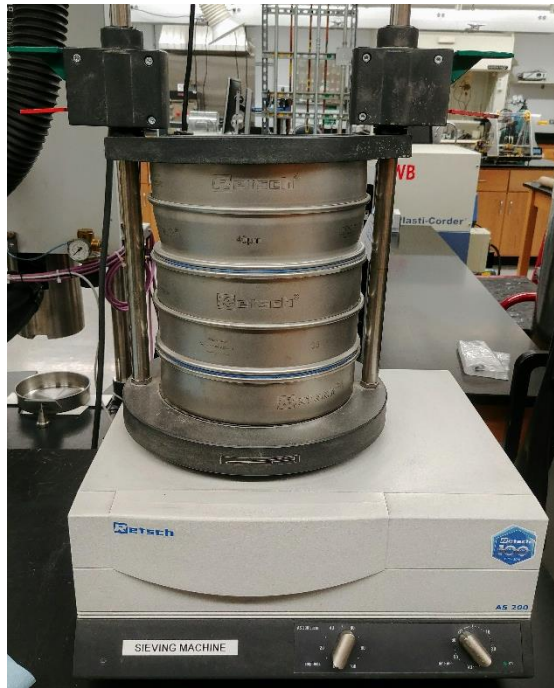
Figure A.5 Retsch AS 200 machine was used for vibratory sieving of the as-received fine 420 stainless steel powder.
