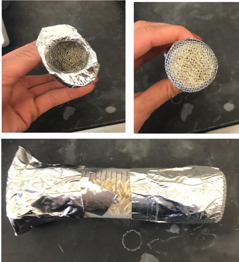
Figure 33: Test rig for the extrudates, using a modified syringe
