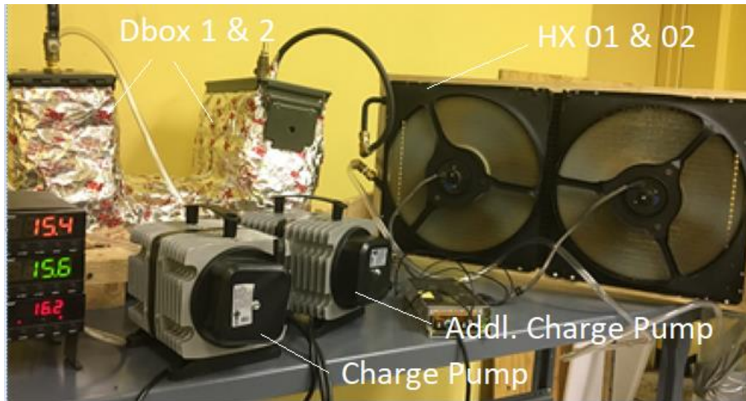
Figure 38: Use of a car intercooler as the condenser
