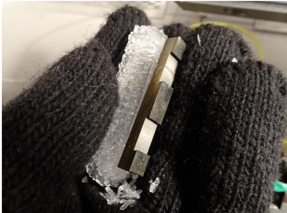
Figure 58. Sample W13 showed relative motion between the ice and coupon and was bonded on removal.
