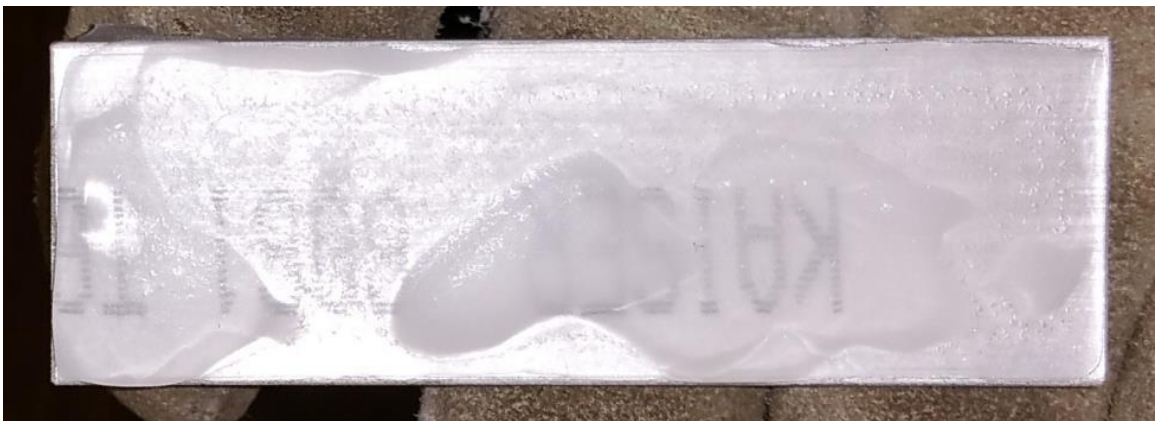
Figure 21. Ice created using pipette on sub-freezing aluminum sample, 1"x3".
