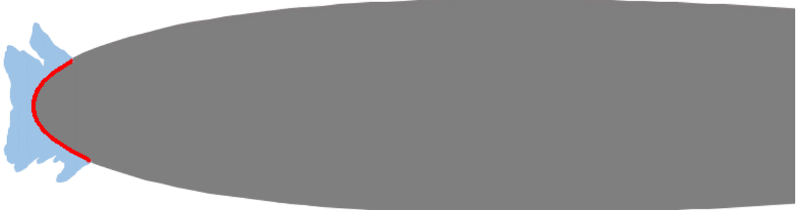
Figure 43. Illustration of A and W variables. A is the cross-sectional area of the ice (light blue area), and W is the length of the red line. Gray area is a cropped NACA 0012 airfoil.
