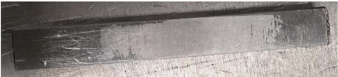
Figure 78. Sample AB10 post-test showing frost in the middle of the sample.
