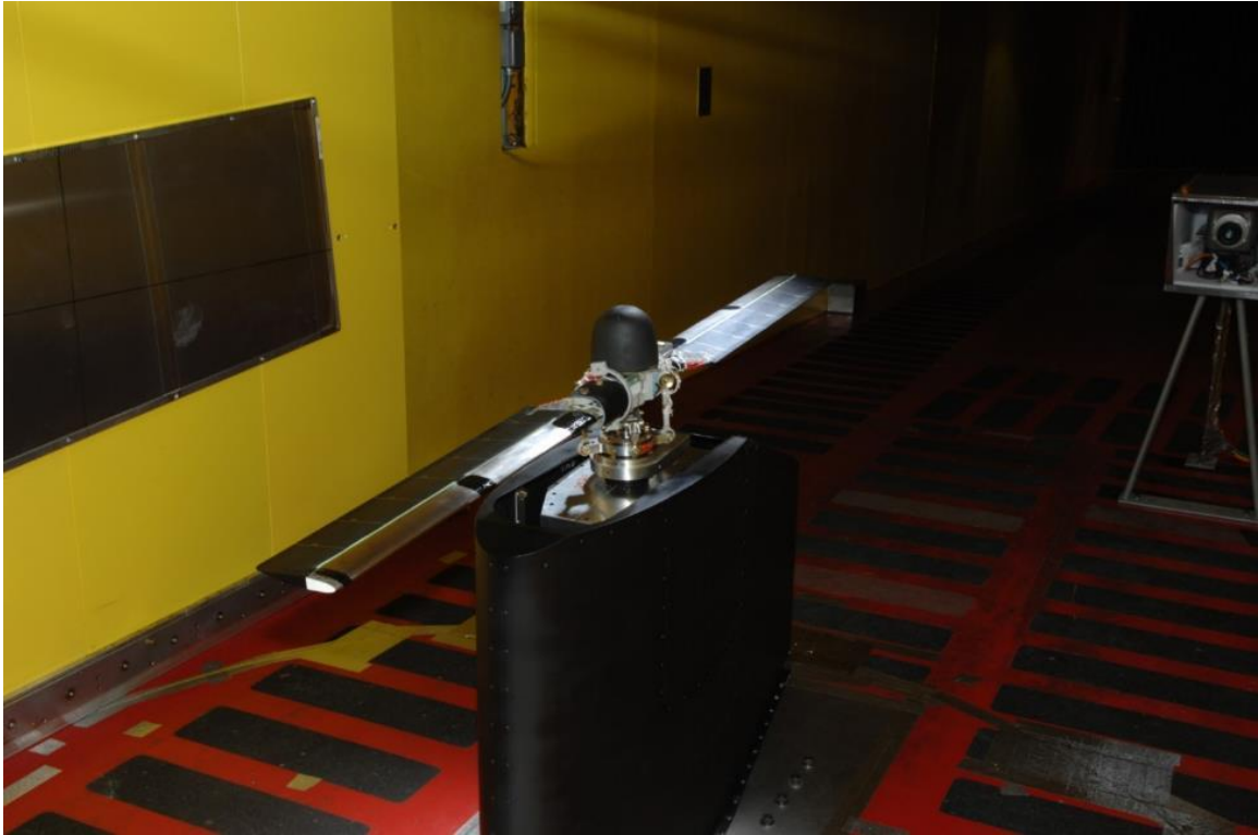
Figure 38. Rotor stand inside test section of IRT in 2013 tests [168].
