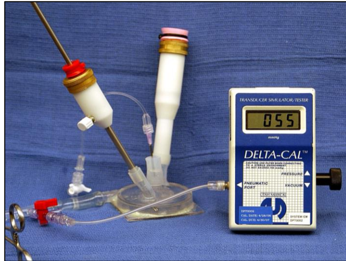
Figure 32 – Benchtop leak test setup
