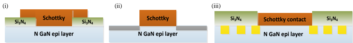
Figure 2-11: Common field termination techniques (i) field plate design (ii) damage implant (iii) guard-ring using p implants
