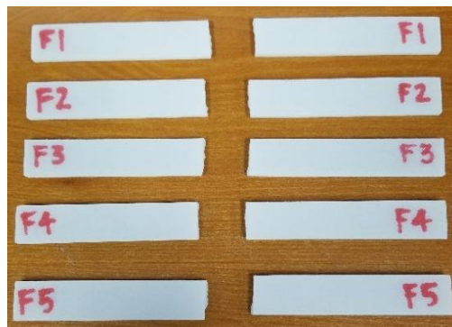
FIGURE 40. Flexural test specimens for the 45%GF blend.
