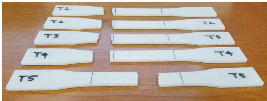
FIGURE 36. 35%GF blend tensile test specimens. All specimens except for specimen 5 had failed outside of the gauge length. The dark lines represent the placement of the extensometer during testing.
