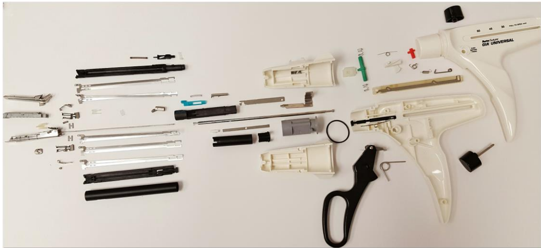
Figure 20. Covidien Endo GIA™ Universal stapler and the Covidien Endo GIA™ Universal Roticulator™ reload exploded view.
