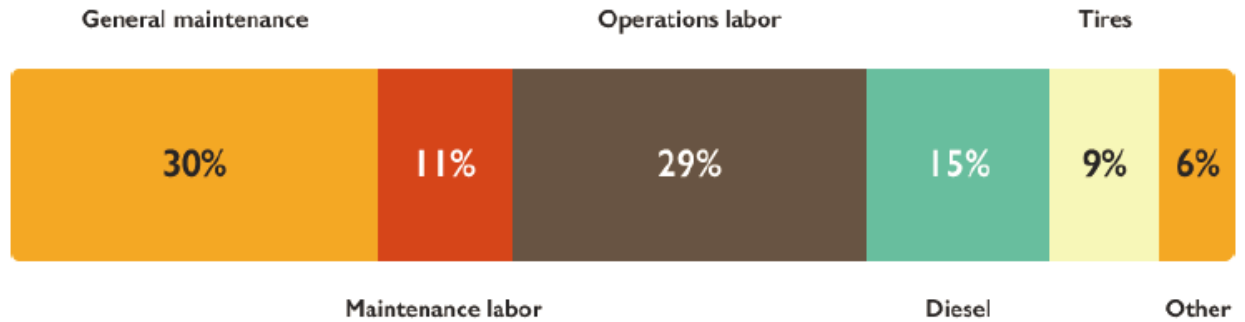
Figure 4- Breakdown of direct mining costs in large open pit mines in the US (Fekete, 2015)
