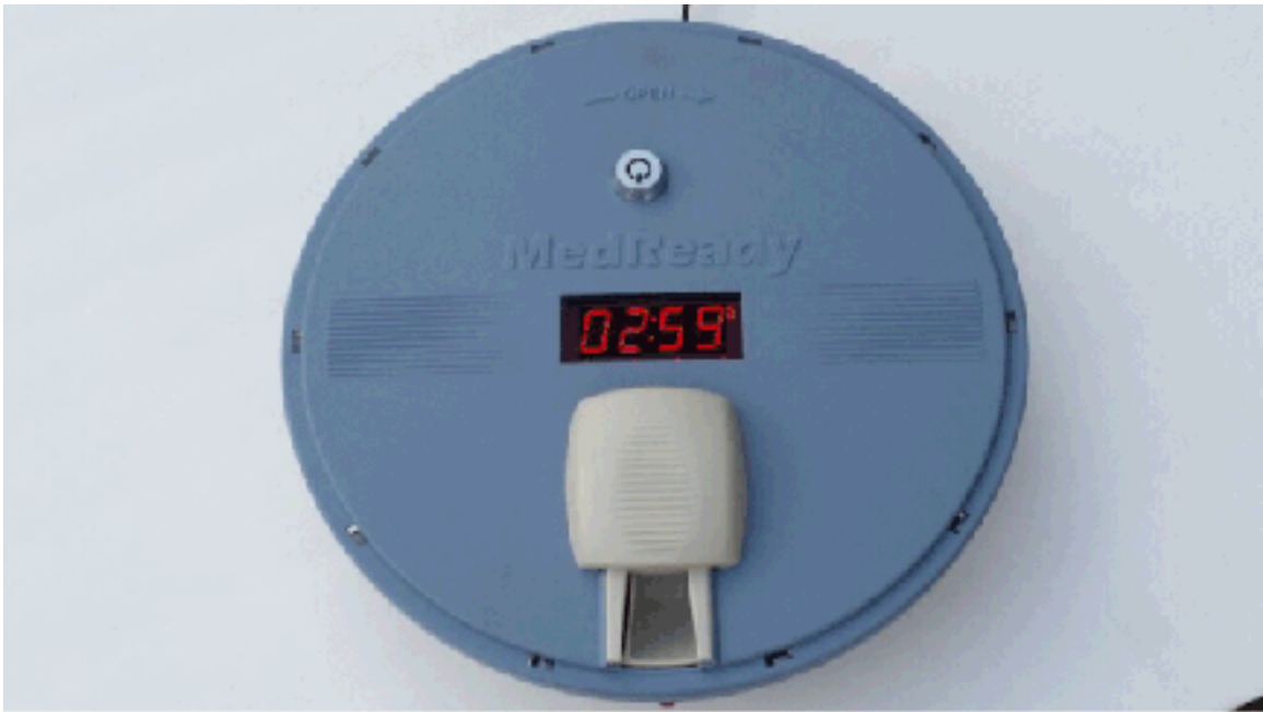
FIGURE 9. MEDREADY MMD BY MEDREADY, INC. TOP-DOWN VIEW SHOWS THE PATIENT PERSPECTIVE, AN OPEN COMPARTMENT AND TIME DISPLAY ON LID. IMAGE FROM MEDREADY, INC.
