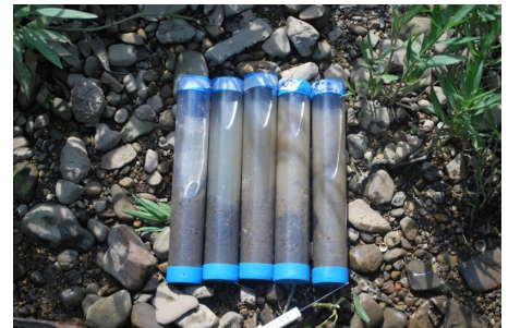
Nate's samples were taken to the lab and sorted with the fine sediments (after weighing), then going to Hayley for sediment chemistry analysis.
