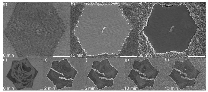
**Figure 2.26.** SEM images of graphene domains before treatment (0 min) and after repeated  $H_2S$  treatment. The total amount of  $H_2S$  treatment time is denoted in each SEM image. Cracks can be visualized with formation of  $Cu_2S$  nanoparticles in the crack regions. **(a-c)** Two cracks originate from domain center, resembling hour and minute hands in a clock. **(d-h)** Branched cracks. Scale bar:  $2 \mu m$ .
