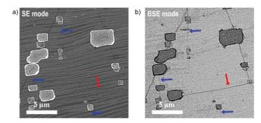
**Figure 3. 5. (a)** An SEM image of the graphene on copper surface after dipping in an aqueous HCl solution for 10 minutes. **(b)** BSE mode image of the same region in (a). Blue and red arrows indicate wrinkles in the images.<sup>19</sup>
