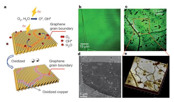
**Figure 1.10.** Observation of graphene grain boundaries after ultraviolet exposure under moisture-rich ambient conditions. **(a)** Schematic of the ultraviolet treatment of a graphene on copper sample. **(b,c)** Optical images of graphene on copper before **(b)** and after **(c)** oxidation. **(d)** SEM image of oxidized graphene on copper. **(e)** AFM image of the location marked by a red square in **(c)**.<sup>51</sup>
