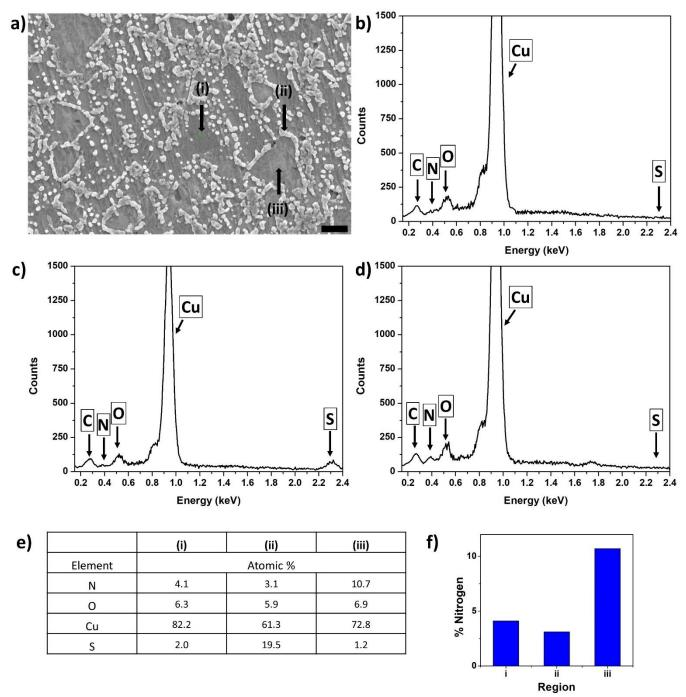
**Figure 4.7.** EDX spectra of h-BN on copper after H<sub>2</sub>S gas treatment for 2 minutes. **(a)** SEM image of monolayer h-BN on copper with newly formed particles. The scale bar: 0.5 μm. **(b,c,d)** EDX spectra of spots indicated as **(i)**, **(ii)** and **(iii)** in **(a)** in order, respectively. **(e)** Table showing the elemental composition of the analyzed spots in (a) by atomic percentage. **(f)** Bar graph for atomic percentage of nitrogen in regions i, ii and iii in (a).
