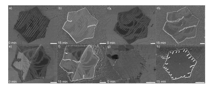
**Figure 2.13.** SEM images of graphene domains before and after  $H_2S$  treatment. Both kinked and straight cracks can be visualized with formation of  $Cu_2S$  nanoparticles in the crack regions. Scale bar:  $2 \mu m$ .
