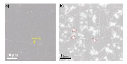
**Figure 4.3.** SEM images of CVD grown h-BN on copper foil. **(a)** Low-magnification SEM image of a continuous monolayer h-BN. The yellow arrow indicates one of the h-BN wrinkles. **(b)** Higher magnification image, showing triangular multilayer pyramidal h-BN islands (some of which indicated with red triangles) on monolayer h-BN.<sup>25</sup>
