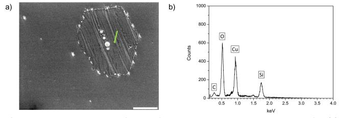
**Figure 2.7.** Elemental analysis of particle found on the graphene domain on copper foil. **(a)** EDS beam is focused on the center of the particle on a graphene domain that is indicated by the arrow in the SEM image. **(b)** The EDS spectrum of the particle. Scale bar is 2 μm.
