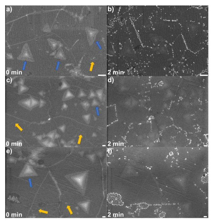
**Figure 4.11**. SEM images of monolayer h-BN on copper foil before **(a,c,e)** and after **(b,d,f)** H<sub>2</sub>S gas treatment. The treatment time is noted on each image. The blue arrows indicate triangular multilayer regions and orange arrows indicate thin or irregular shaped bright regions in **(a,c,e)**, where Cu<sub>x</sub>S particle formation is observed. Scale bar: 0.5 μm.
