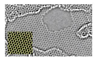
**Figure 1.5.** Aberration-corrected TEM image of a hole in a single layer of graphene. Scale bar:  $5 \text{ Å}.^{37}$
