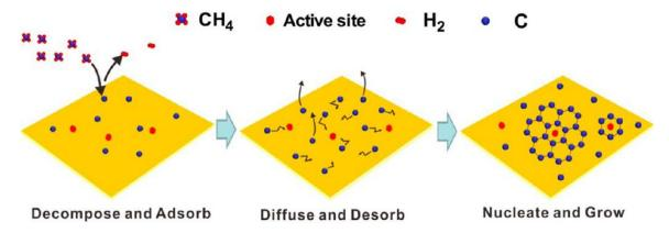
**Figure 1.3.** Illustration of the graphene growth mechanism on copper in CVD process, as divided into three main steps.<sup>19</sup>
