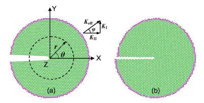
**Figure 2.10.** Boundary layer MD models and coordinates. A pre-existing straight crack along **(a)** zigzag and **(b)** armchair edge is embedded in a two-dimensional graphene lattice (green).  $K_{\text{eff}}$  is effective stress intensity factor.  $K_{\text{I}}$  and  $K_{\text{II}}$  are SIF components specified by opening and shear stress, respectively.  $\varphi$  is the phase angle.<sup>11</sup>
