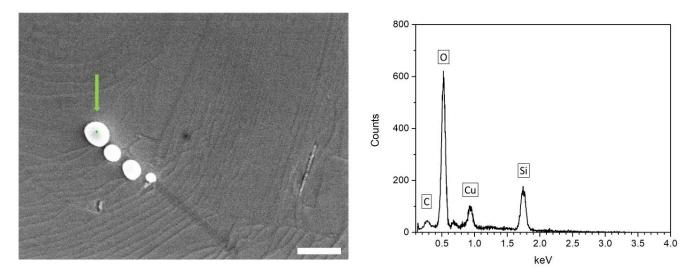
**Figure 2.18.** EDX spectrum (right) of a pre-existing nanoparticle in polycrystalline graphene film before the H<sub>2</sub>S treatment. Electron beam was focused on the center of the nanoparticle (indicated by the green arrow) in the SEM image (left). Scale bar: 0.5 μm.
