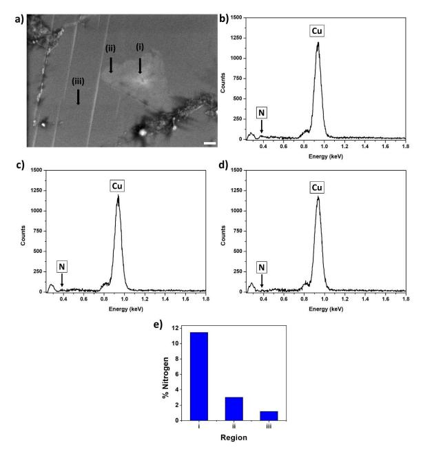
**Figure 4.6.** EDX spectra of pristine h-BN on copper. **(a)** SEM image of monolayer h-BN on copper with a triangular multilayer region. The scale bar: 0.2 μm. **(b,c,d)** EDX spectra of spots indicated as **(i)**, **(ii)** and **(iii)** in **(a)** in order, respectively. **(e)** Bar graph for atomic percentage of nitrogen in regions i, ii and iii in **(a)**.
