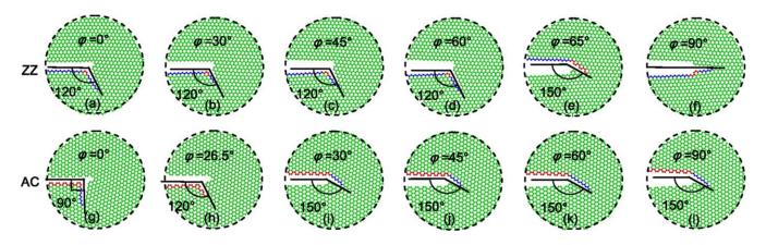
**Figure 2.11.** The crack propagation after initiation in Figure 2.10 under complex mechanical stress. **(a–f)** Zigzag (ZZ) crack models at  $\varphi$ = 0°, 30c, 45°, 60°, 65°, and 90°. **(g–l)** Armchair (AC) crack models at  $\varphi$ = 0°, 26.5°, 30°, 45°, 60°, and 90°, respectively. The angle of crack propagation orienting to primary crack is depicted correspondingly. ZZ crack edges are shown in blue, AC in red.<sup>11</sup>
