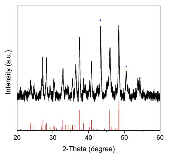
**Figure 2.6.** XRD pattern of Cu<sub>2</sub>S nanoparticles scraped off from the copper foil surface. The asterisks indicate diffraction peaks coming from copper particles.
