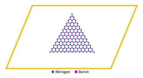
Figure 4.1. Illustration of atom arrangement of monolayer triangular h-BN domain.
