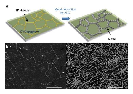
**Figure 1.8.** Visualization of one-dimensional defects in CVD-grown graphene by ALD. **(a)** Schematic of selective Pt growth on various line defects such as grain boundaries, cracks and folded structures in CVD graphene. **(b)** SEM image of graphene on a glass substrate after 500 ALD cycles of Pt deposition. **(c)** SEM image of graphene with Pt deposition after 1000 ALD cycles. Scale bar:  $2 \mu m$ .<sup>49</sup>
