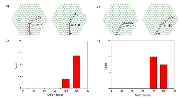
**Figure 2.14. (a,b)** Schematic illustration of representative kinked graphene crack structures. **(c)** Histogram of the distribution of kink angles ( $\theta$ ) for the cracks starting at 90° ( $\pm$  10°) angle ( $\alpha$ ) from zigzag edge. **(d)** Histogram of the distribution of kink angles ( $\theta$ ) for the cracks starting at 60° ( $\pm$  10°) or 120° ( $\pm$  10°) angle ( $\alpha$ ) from zigzag edge.
