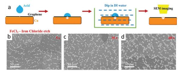
**Figure 1.11. (a)** Schematic illustration of the under-etching process for CVD-grown graphene on copper foil. SEM images showing the etch pits formed after iron chloride solution etch for **(b)** 5 s, **(c)** 30 s, **(d)** 60 s.<sup>60</sup>
