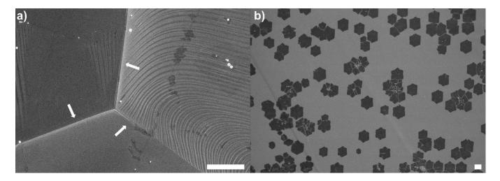
**Figure 2.2.** Representative SEM images of the purchased CVD-grown graphene on copper. (a) The pristine continuous graphene film from the front side of the sample. The white arrows indicate copper grain boundaries. (b) Pristine multiple hexagonal graphene domains as well as coalesced domains from the back side of the sample. Scale bar: 20 μm.
