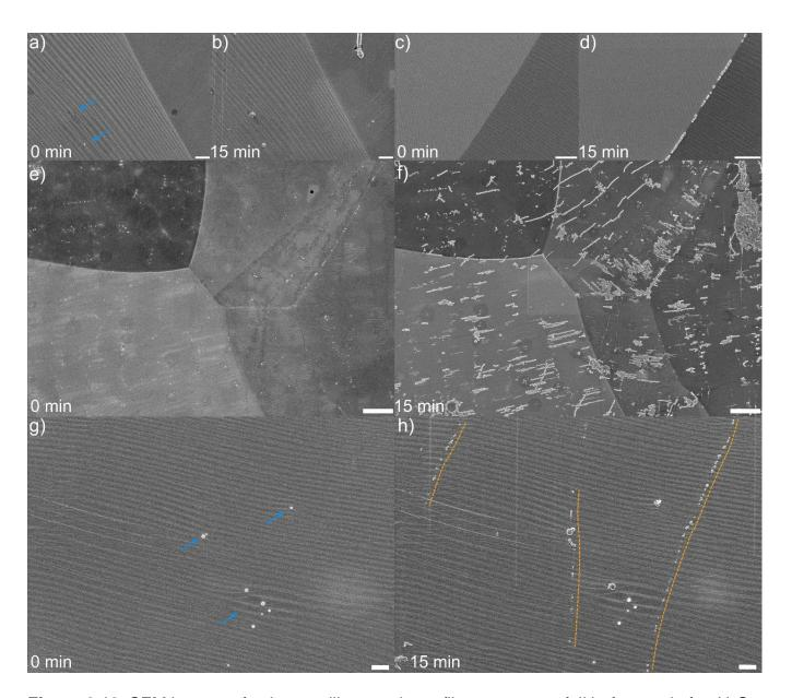
**Figure 2.19.** SEM images of polycrystalline graphene films on copper foil before and after H<sub>2</sub>S gas treatment. **(a,b)** Cu<sub>2</sub>S nanoparticles emerge from both SiO<sub>x</sub> nanoparticle sites (indicated
