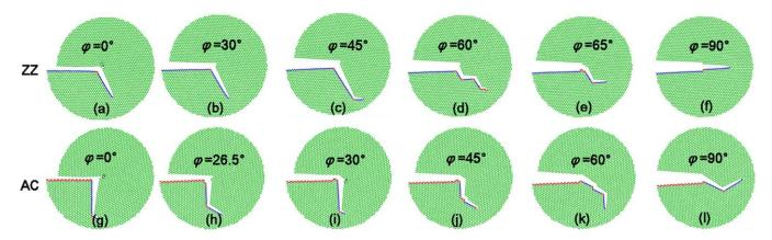
**Figure 2.12.** Images of crack kinking in graphene lattices (green) after propagation in Figure 2.11. ZZ (blue), or AC (red) edges appear alternatively changing direction of growth.<sup>11</sup>
