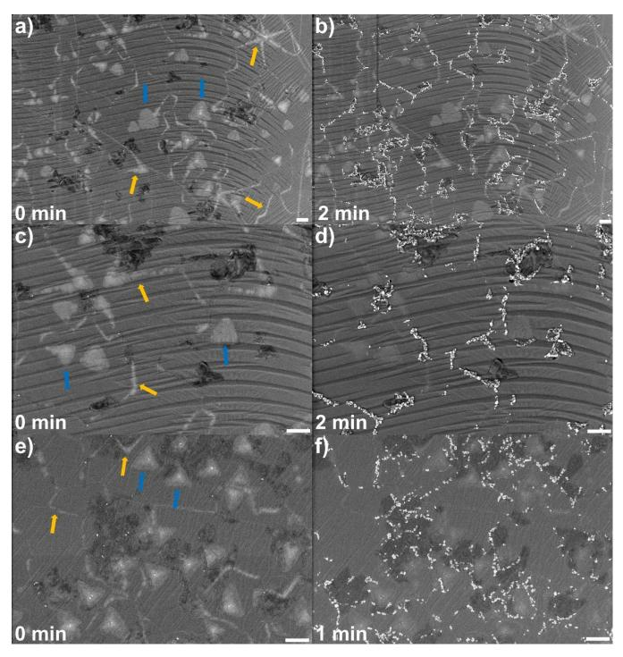
**Figure 4.8.** SEM images of monolayer h-BN on copper foil before and after  $H_2S$  gas treatment. **(a,b)** SEM images of the same region before and after 2 min treatment. **(c,d)** The higher magnification images of the upper-middle region in **(a)**. **(e,f)** SEM images of another region before and after 1 min  $H_2S$  gas treatment. Scale bar: 0.5  $\mu$ m.
