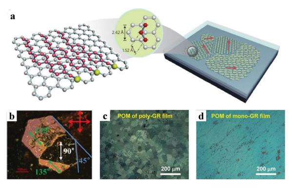
**Figure 1.9. (a)** Schematic of liquid crystal alignment on the surface of the graphene. The alignment directions of liquid-crystal molecules depend on the orientations of graphene domains. **(b)** POM images of graphene islands coated with liquid-crystal molecules on glass. **(c,d)** POM images of polycrystalline and monocrystalline graphene films coated with liquid-crystal molecules on a Cu substrate, respectively.<sup>45</sup>
