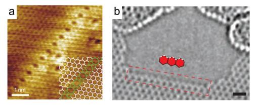
**Figure 1.7. (a)** STM image of a grain boundary in graphene. Scale bar: 1 nm.<sup>33</sup> **(b)** Aberration corrected TEM image of a hole in a single layer of graphene. Scale bar: 5 Å.<sup>37</sup>
