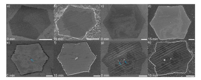
**Figure 2.8.** SEM images of monolayer hexagonal graphene domains on copper foil before and after  $H_2S$  gas treatment. **(a,b)** No  $Cu_2S$  nanoparticle is detected after  $H_2S$  treatment. **(c,d)**  $Cu_2S$  nanoparticle is formed only at the nucleation center of graphene domain. **(e-h)**  $Cu_2S$  nanoparticles emerge from  $SiO_x$  nanoparticle sites (indicated by blue arrows) after  $H_2S$  treatment. Scale bar:  $2 \mu m$ .
