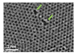
**Figure 4.9.** HRTEM image of CVD-grown h-BN with vacancy defects at the grain boundary region indicated by green arrows.<sup>33</sup>
