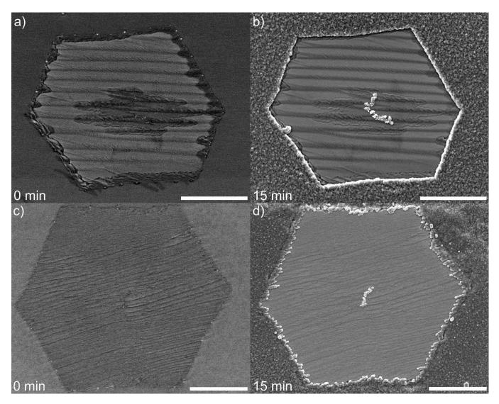
**Figure 2.16.** SEM images of graphene domains before **(a,c)** and after **(b,d)**  $H_2S$  treatment. Two cracks originate from domain center, resembling hour and minute hands in a clock. Scale bar: 2  $\mu$ m.
