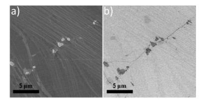
**Figure 3.4. (a)** SEM image of monolayer graphene on copper film. The subtle surface features such as graphene wrinkles are not obvious. **(b)** SEM-BSE image of the same region in **(a)**. The graphene wrinkles that are not visible or partially visible in **(a)** are obvious. <sup>19</sup>
