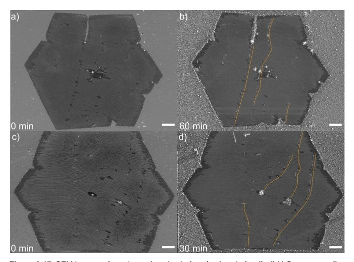
Figure 2.17. SEM images of graphene domains before (a,c) and after (b,d) H<sub>2</sub>S treatment. (b-d) Discontinuous cracks highlighted by orange dashed lines. Scale bar: 3  $\mu$ m.
