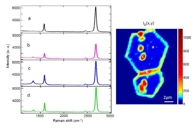
**Figure 1.6.** Individual Raman spectra taken from 4 representative locations on graphene (left). Spectroscopic Raman mapping of graphene grains and grain boundary (right). (a) inside a single crystalline graphene grain, (b) on the grain boundary location, (c) on a defect site, which could be a nucleation center, inside an individual grain, and (d) on the edge of graphene.<sup>40</sup>
