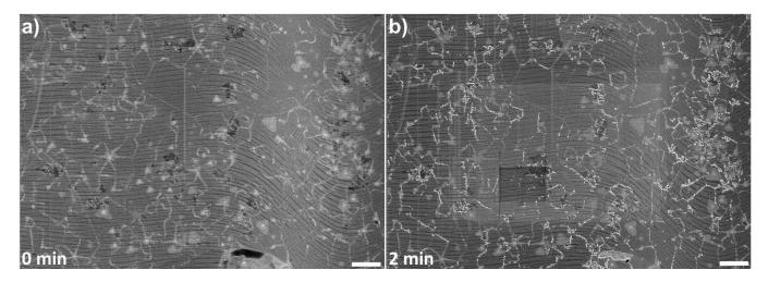
**Figure 4.10.** SEM images of monolayer h-BN on copper foil before and after 2 minutes of  $H_2S$  gas treatment. Scale bar: 2  $\mu$ m.
