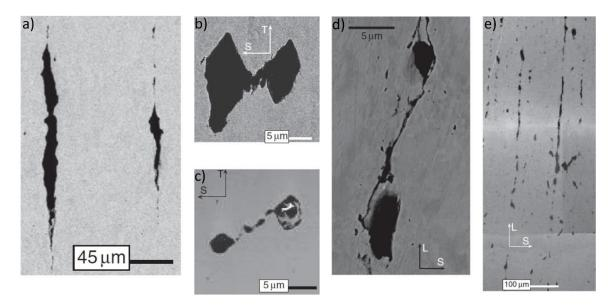
**Figure 2.21.** (a) Void growth. (b-e) Modes of void coalescence: (b) Necking of intervoid ligament (c-d) Coalescence in a microshear band. (e) "Necklace" coalescence.<sup>21</sup>
