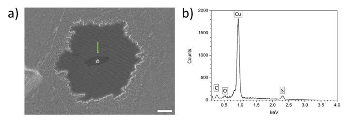
**Figure 2.5.** EDX spectrum **(b)** of a nanoparticle formed on graphene domain after the  $H_2S$  treatment. Electron beam was focused on the center of the nanoparticle (indicated by the green arrow) in the SEM image **(a)**. Scale bar: 3  $\mu$ m.
