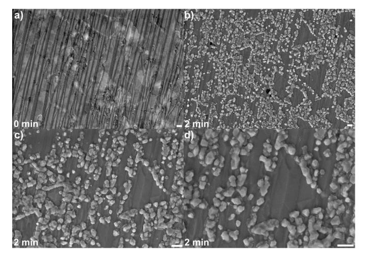
**Figure 4.12**. SEM images of monolayer h-BN on copper foil before and after H<sub>2</sub>S gas treatment. **(a,b)** SEM images of the same region before and after 2 min treatment, respectively. **(c,d)** The higher magnification images of the upper-right region in **(a)**. Scale bar: 0.2 μm.
