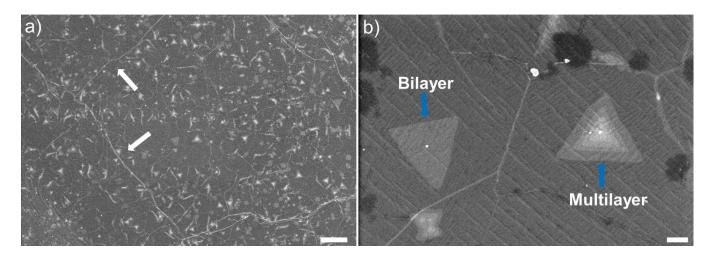
**Figure 4.5.** SEM images of CVD grown h-BN on copper foil. **(a)** Low-magnification image, showing excessive multilayers of h-BN in monolayer h-BN. The white arrows show the wrinkles on h-BN. **(b)** High-magnification image in the same region, showing triangular adlayer and multilayer pyramidal h-BN island on monolayer h-BN. Scale bar: **(a)** 2 μm and **(b)** 0.2 μm.
