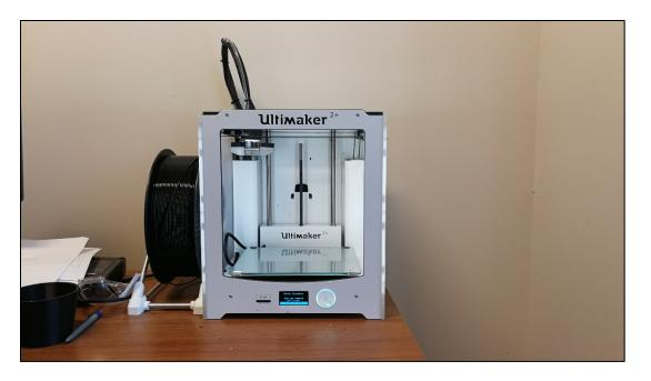
Figure 26: Ultimaker 2+ 3-D printer
