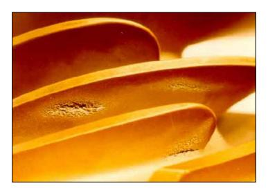
Figure 4: Localized cavitation damage on a pump blade [9]
