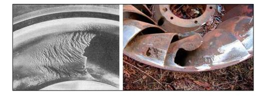
Figure 5: Severe cavitation erosion as witnessed on a Francis turbine [10]
