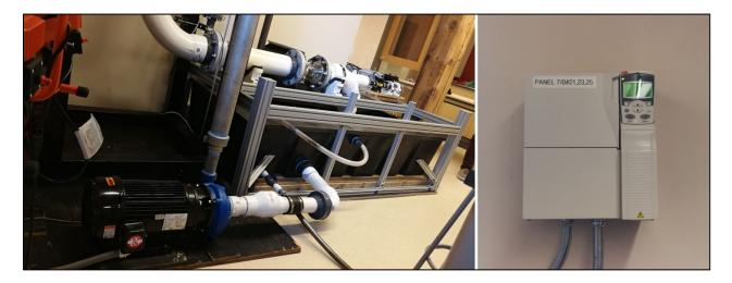
Figure 31: Pump-motor set and VSD
