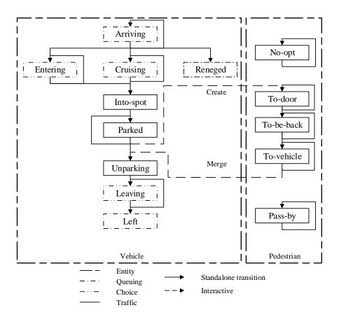
Figure 4-19 Parking simulation entity process transition
