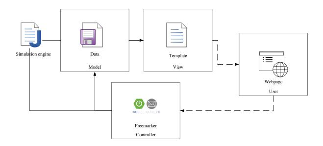
Figure 3-11 The server-side application structure
