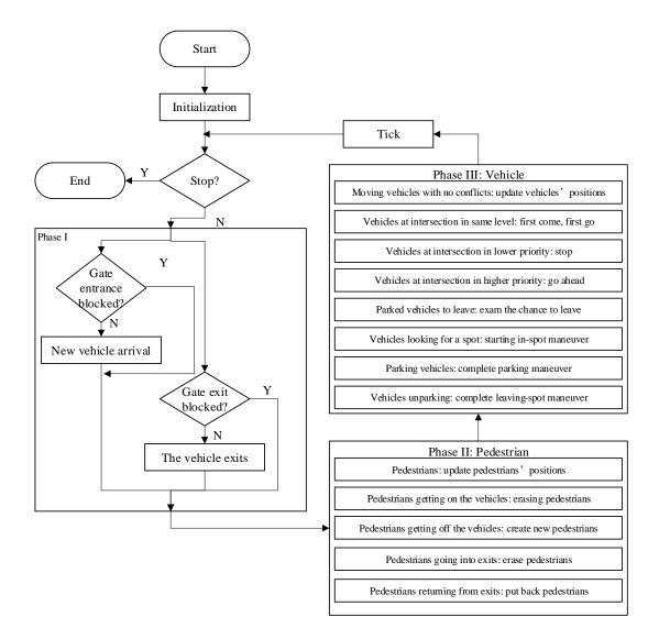
Figure 3-2 The proposed simulation procedure for off-street parking facilities
