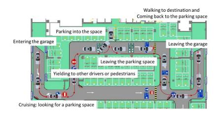
Figure 3-1 A sample parking process
