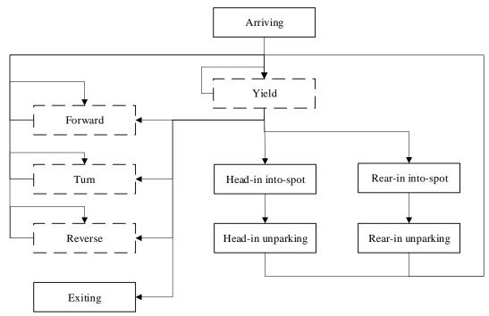
Figure 4-20 Vehicle movement behavior modeling diagram
