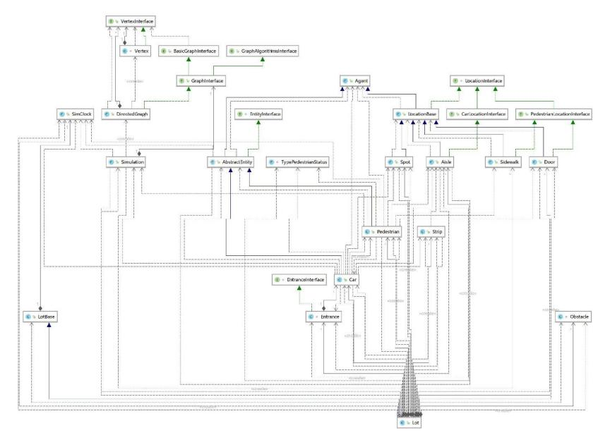
Figure 3-8 The class diagram of the core of the simulation engine in UML
