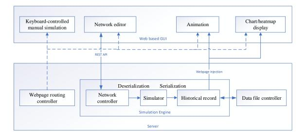
Figure 3-10 The software architecture of the proposed SaaS system
