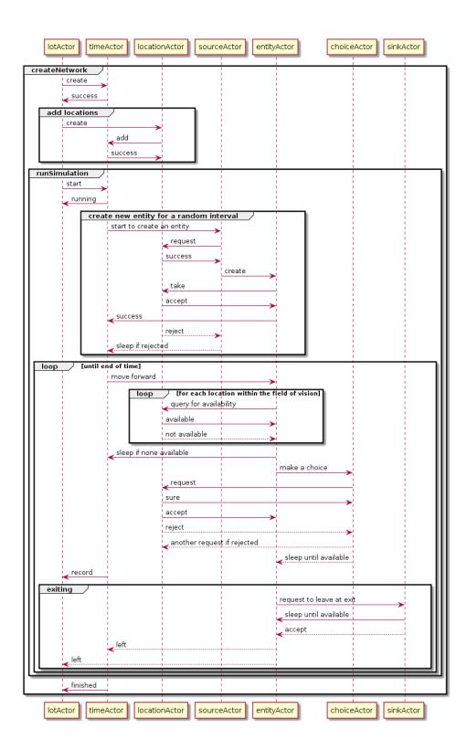
Figure 3-9 The sequence diagram in Unified Marked Language
