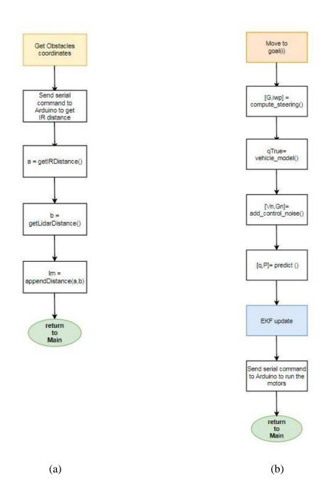
Figure 20: (a) Flowchart to get Obstacle coordinates (b) Flowchart to move the robot to a desired goal
