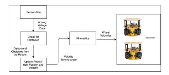
Figure 18: Controls structure
