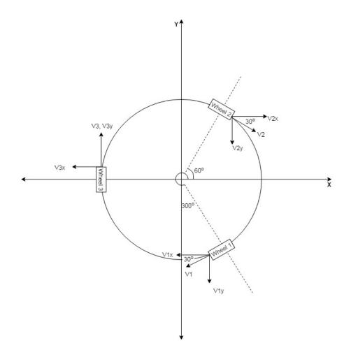
Figure 3: Wheel vector analysis for Omni-wheeled drive
