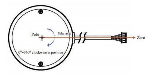
Figure 14: Lidar Configuration diagram
