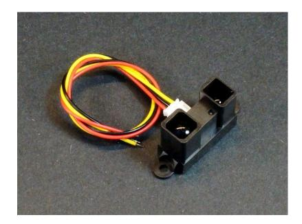
Figure 10: GP2Y0A02YK0F IR Sensor
