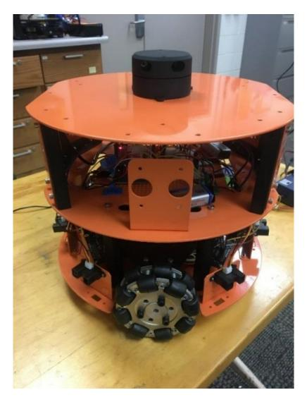
Figure 7: HCR Omni wheeled robot with LIDAR
