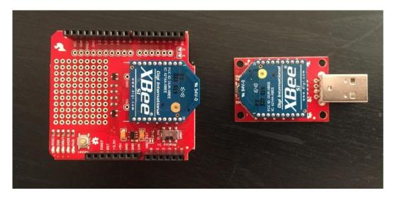
Figure 9: XBee S1 modules with Sparkfun Arduino Shield (Left) and USB Adapter (Right)
