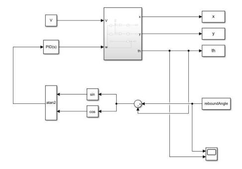
Figure 22: Simulink for PID Control
