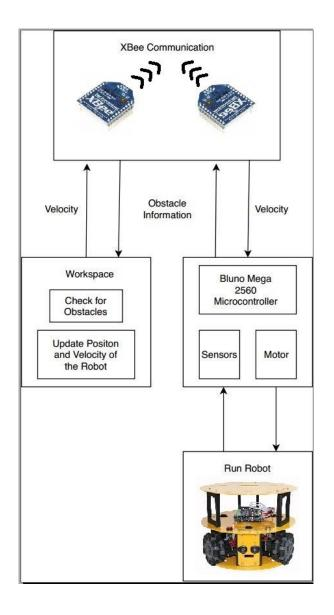
Figure 16: Hardware Setup
