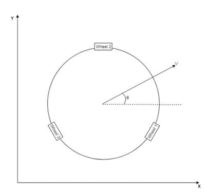
Figure 2: Rotation with respect to the robot center
