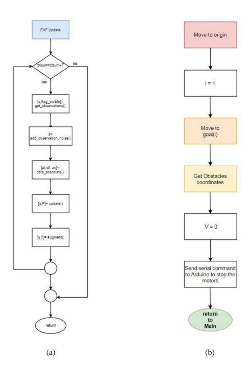
Figure 21: (a) Flowchart to update coordinates (b) Flowchart to move the robot to the origin
