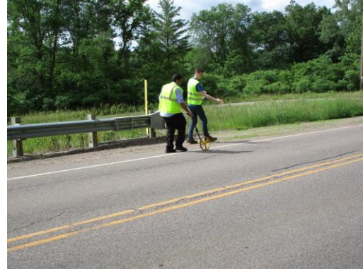
(b) Measuring distresses
