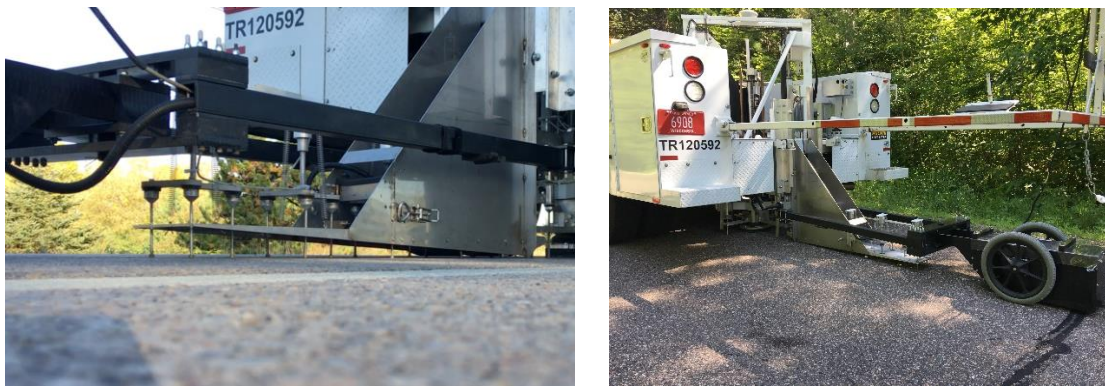
(a) FWD plate and sensors on pavement surface
