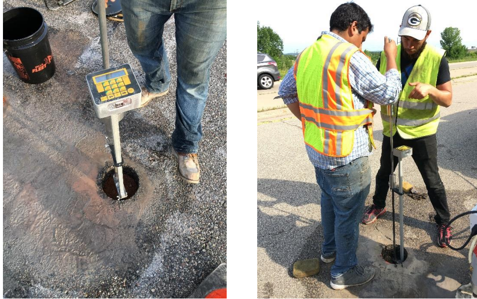
Figure 3.5: Dynamic cone penetration test on aggregate base course layers.
