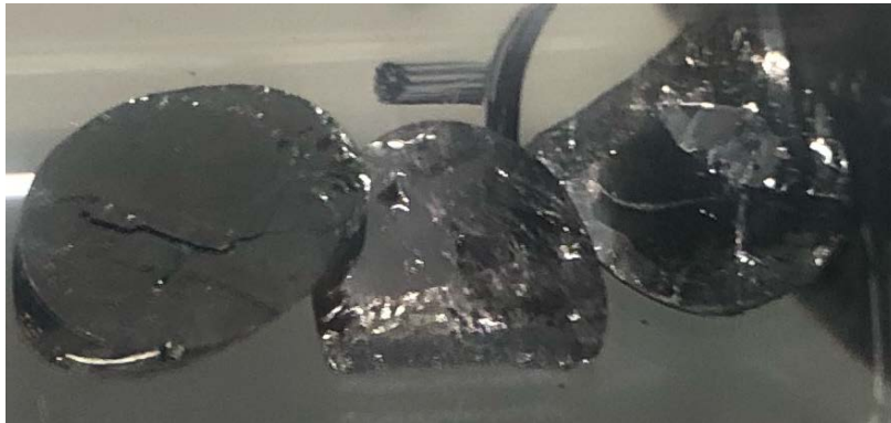
Figure 2-1. Single crystals of iron telluride
