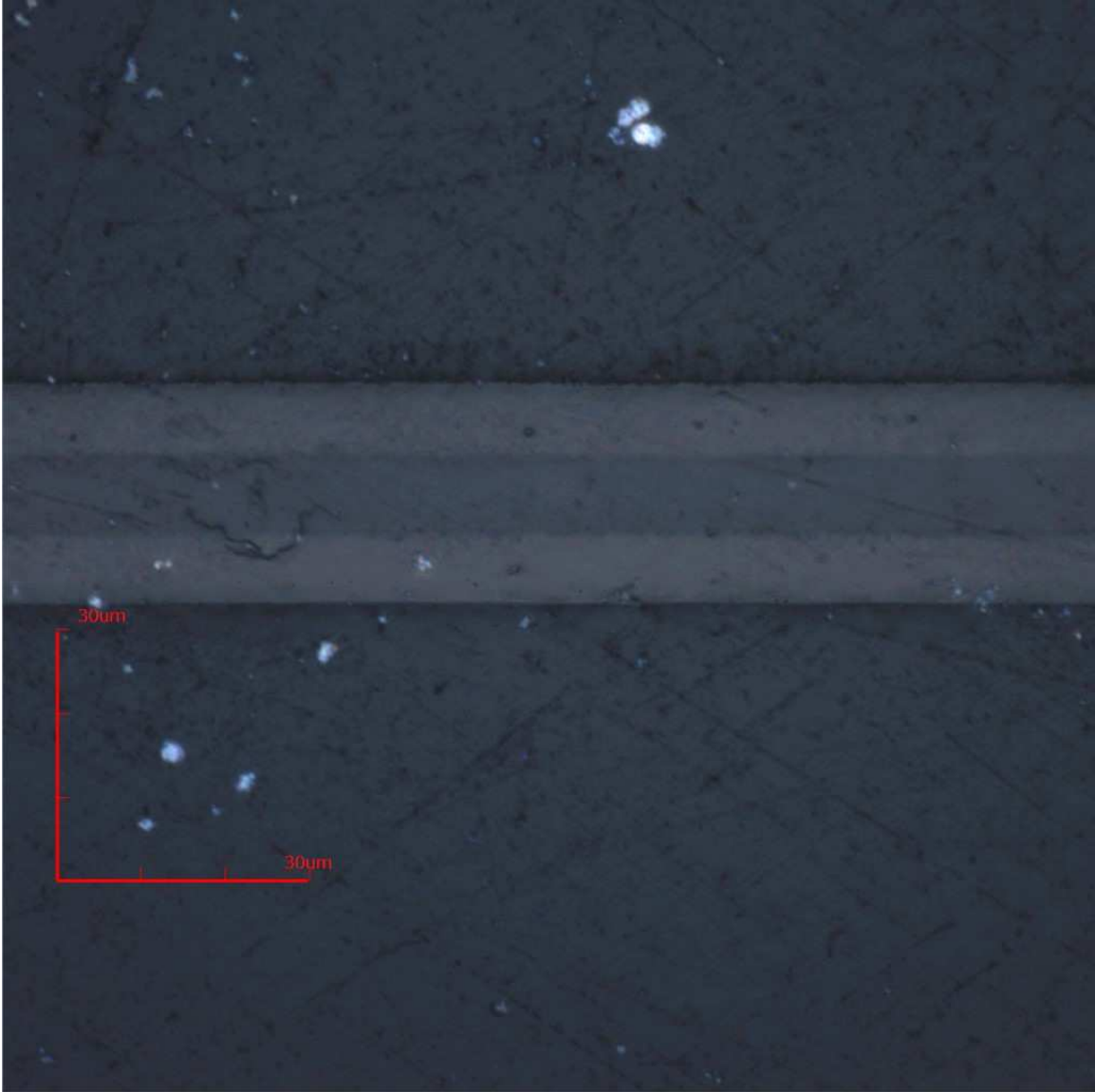
Figure 12: 3-D Microscopy Cross-Section of 110°C Separator
