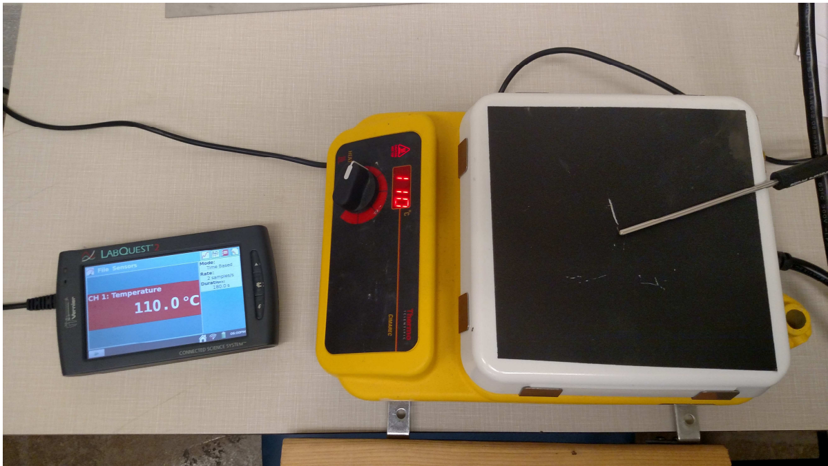
Figure 4: Hotplate with Thermal Couple
