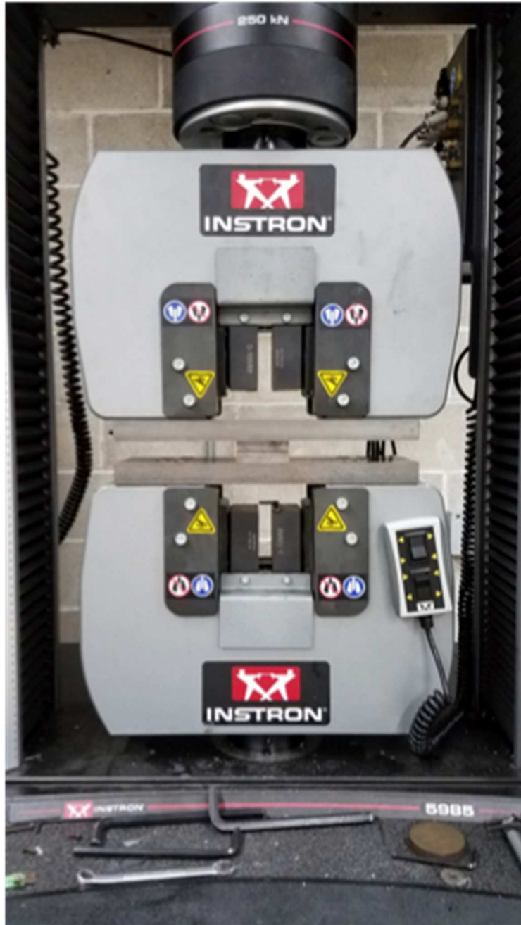
Figure 3: Separator Loading Setup Between Two Flat Plates Using Instron 5985
