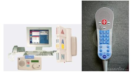
Figure 2. Critical Alert Nurse Call System Components
