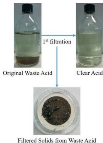
Figure 5-4 Raw waste acid pretreatment. Original waste acid was filtrated for later metal ion separation. Filtered solids were introduced to lead material refinement.
