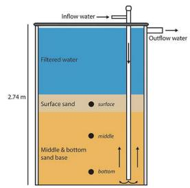
Figure 3.1 Illustration of UWM Biofilter Cross-Section
