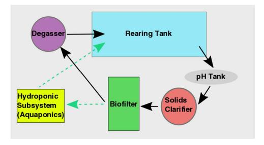
Figure 2.1 - Generalized System Diagram of All Components Sampled
