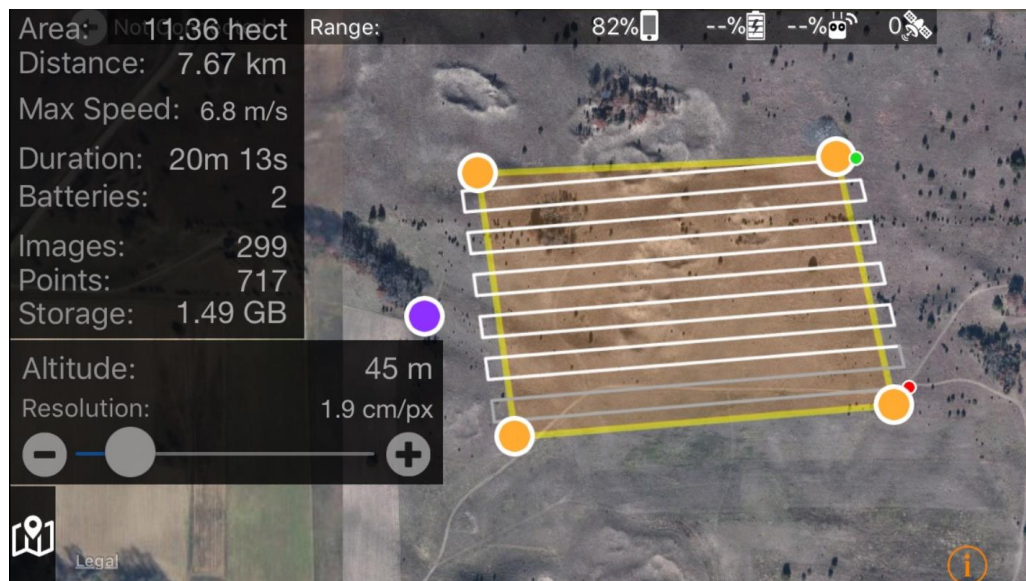
Figure 2. A screenshot of the Map Pilot app, used to generate study areas, design flight paths and control photo acquisition. This app runs on a smart phone and controls the drone during flight. The study area is generated by tapping the screen (orange dots). Users control elevation (and, consequently, image resolution). Users also control image overlap (dropdown menu not shown).
