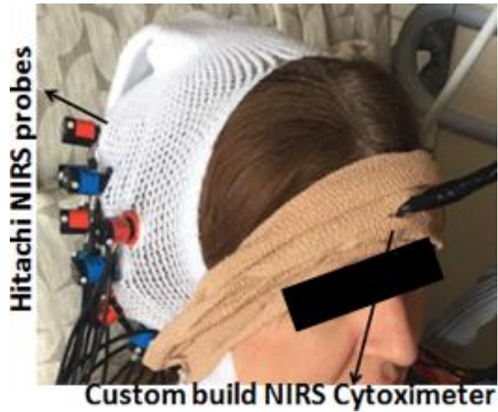
Figure 3.3 Epilepsy protocol, NIRS Cytometer is attached at forehead of the subject and Hitachi NIRS probes are attached at back of the head.
