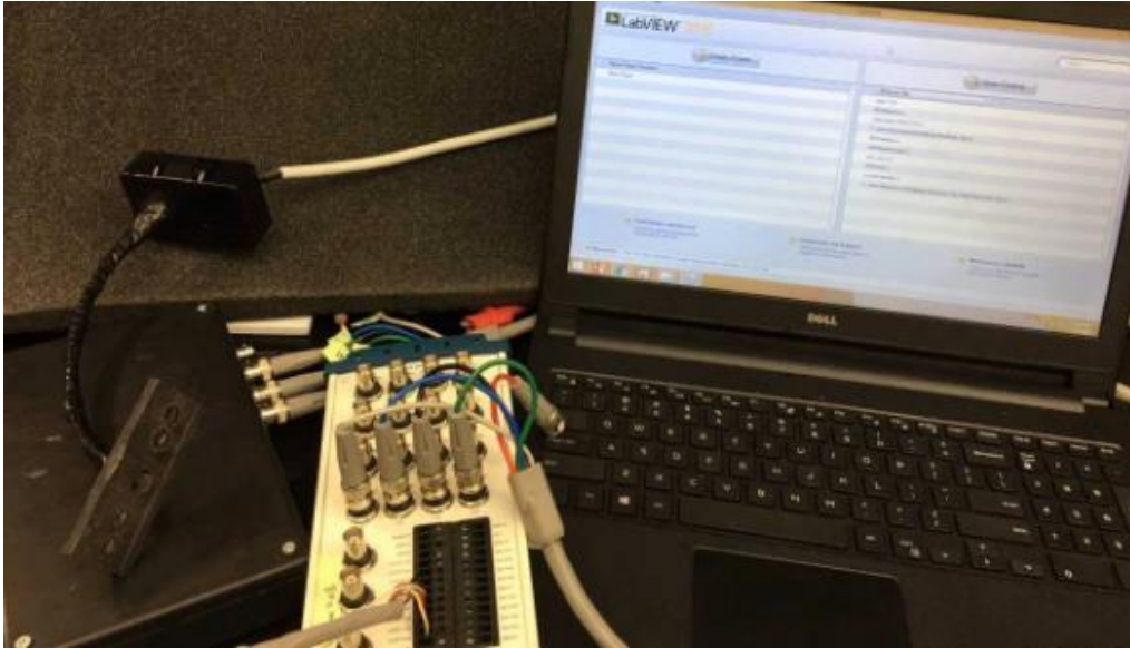
Figure 2.2 Cytoximeter system consists of DAQ board, control box, computer LabVIEW software and probe.
