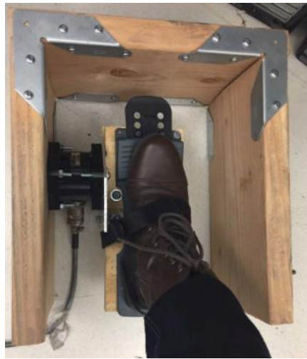
Figure 2.10 The Force plate apparatus, designed to hold the strain gauge which measure the force applied by the subject.
