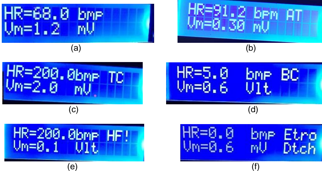
Figure 3.6: (a) normal heart condition; (b) AT: arrhythmia warning; (c) TC: tachycardia warning; (d) BC: bradycardia warning; (e) HF: heart failure warning; (f) Etro Dtch: electrodes not attached warning.
